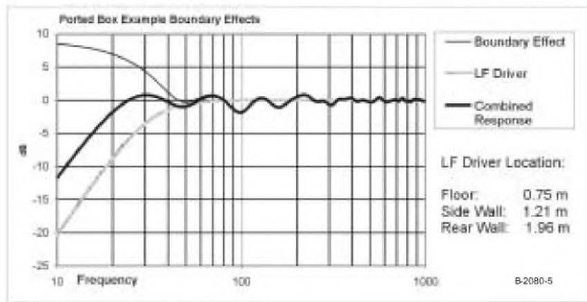
FIGURE 5: MathCAD analysis for ported “optimal” location.
