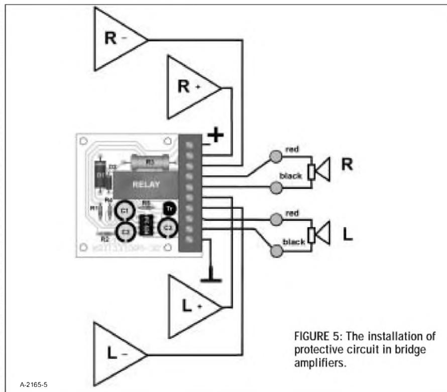
FIGURE 5: The installation of protective circuit in bridge amplifiers.
