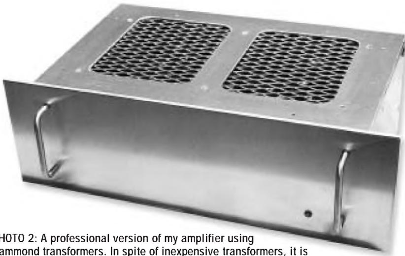
PHOTO 2: A professional version of my amplifier using Hammond transformers. In spite of inexpensive transformers, it is a very good performer.
