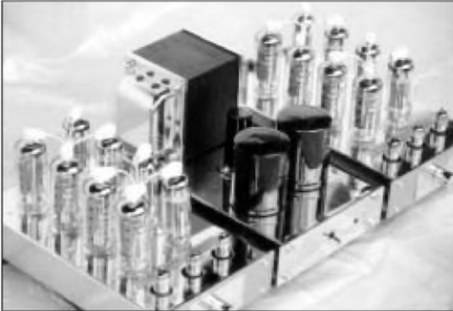
PHOTO 1: The author's version of the Rozenblit 80W transformerless tube output.
