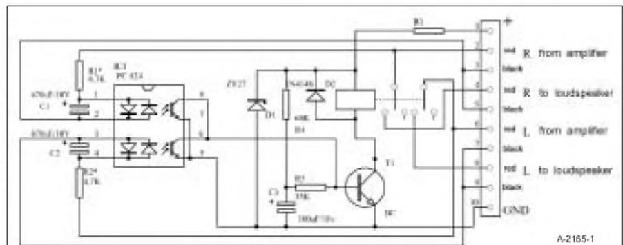
FIGURE 1: The full circuit diagram of the protective circuit. The values of the R1, R2, R3 resistors can vary according to the application. See detailed description.
