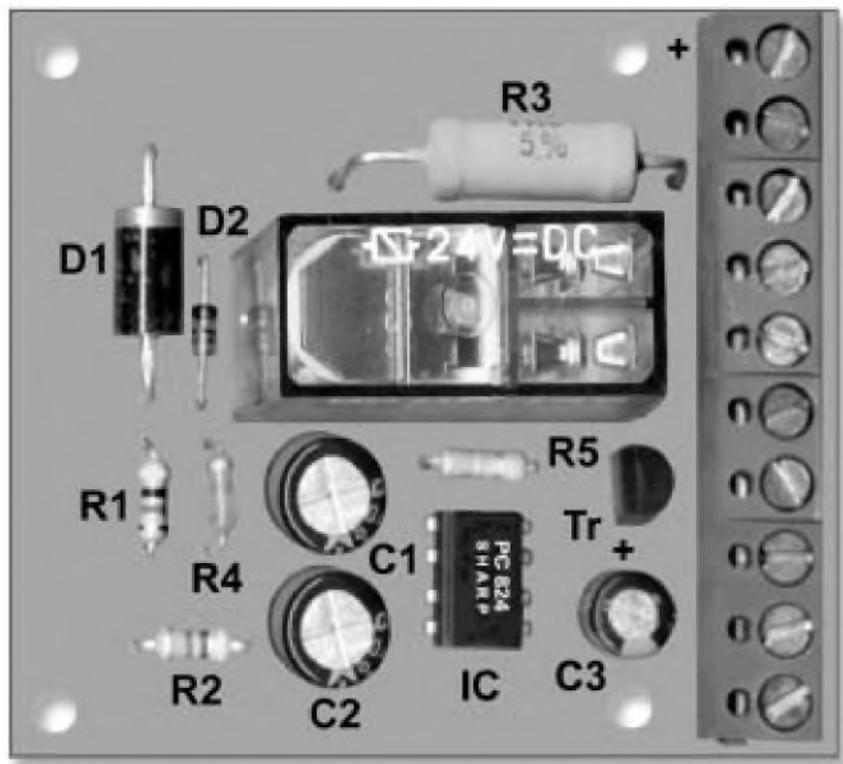
PHOTO 1: The DC protection and switch-on delay circuit.
