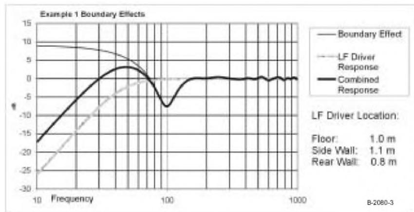
FIGURE 3: MathCAD sealed box  $Q_{TC}$  0.585 analysis first location.
