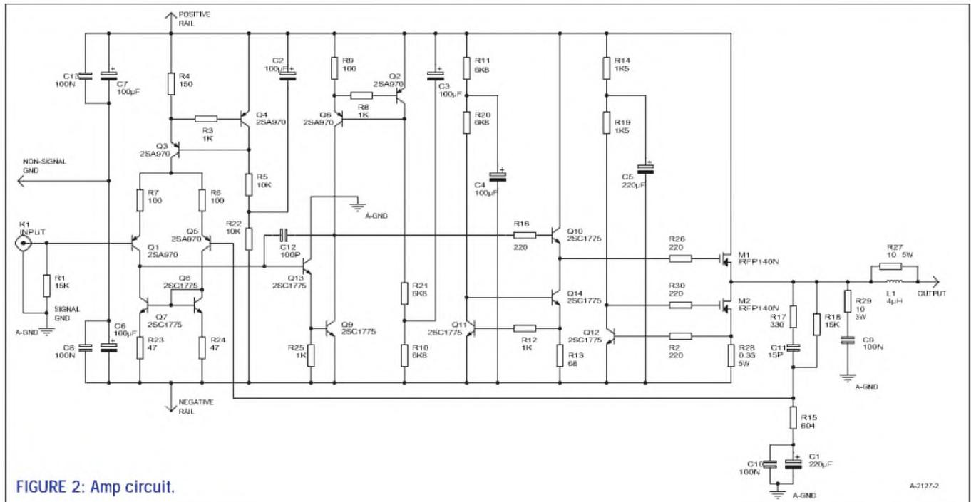
Using the constant-current source discussed earlier,  $.7V/R_x = 2.3A = .313\Omega$ . The nearest available resistor in a 5W package was  $.3\Omega$ . This value caused 2.3A to flow. I now had enough current to give 20W, but I needed to be sure I had enough voltage.
