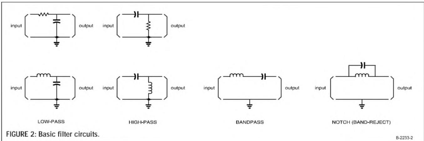
FIGURE 2: Basic filter circuits.
