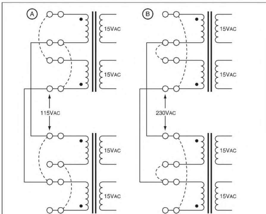
FIGURE 3: Mains transformer wiring for 115V AC mains (3a) and 230V AC mains (3b). The mains frequency (60Hz or 50Hz) is immaterial.
