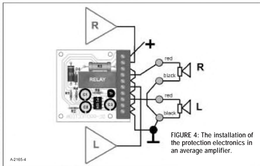
FIGURE 4: The installation of the protection electronics in an average amplifier.
