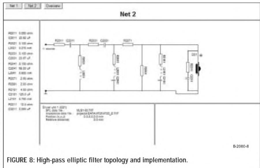
FIGURE 8: High-pass elliptic filter topology and implementation.
