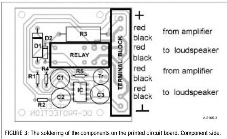
FIGURE 3: The soldering of the components on the printed circuit board. Component side.
