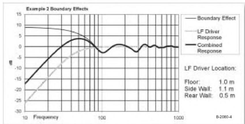
FIGURE 4: MathCAD sealed box  $Q_{TC}$  0.585 analysis second location.
