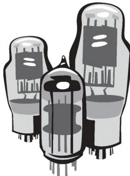
Output tubes such as the 6V6 and 6AC7/EL34 need larger drive voltages. In this case for V2 use a 12AU7, whose much lower internal resistance will provide double the drive that the 12AX7 is capable of. You will need to adapt some of
