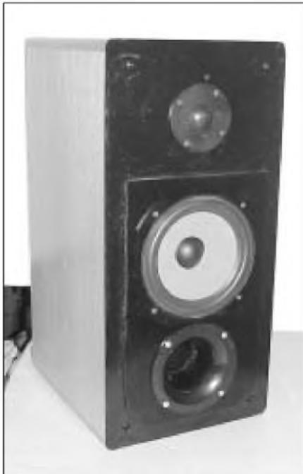
PHOTO 2: The first version, using Focal woofer and MB titanium dome.
