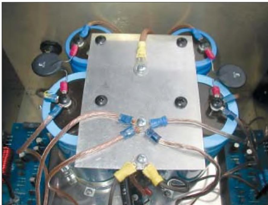
PHOTO 4: Grounding scheme of unit.
