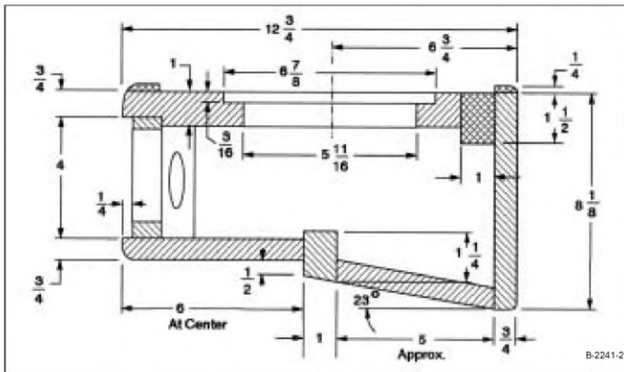
FIGURE 2: Home theater center channel enclosure cross-section.
