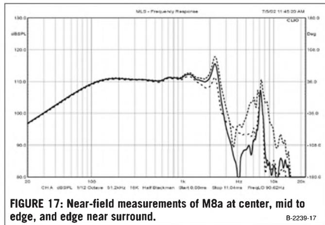
FIGURE 17: Near-field measurements of M8a at center, mid to edge, and edge near surround.
