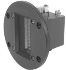
produce sound. In an aluminum ribbon tweeter, the ribbon itself is both the conductive material and the radiating mass moved by the magnet to produce sound. This method results in a wider band width and very smooth phase response. At 0.011 grams, the pure aluminum ribbon has a mass of about 1/20th that of a dome tweeter with comparable surface area.
