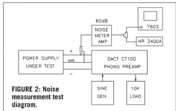
FIGURE 2: Noise measurement test diagram.
