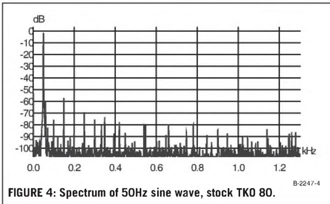
FIGURE 4: Spectrum of 50Hz sine wave, stock TKO 80.
