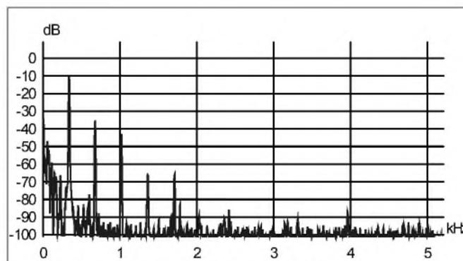
FIGURE 10: Spectrum of bass guitar E, 330Hz.
