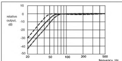
**FIGURE 19: Effects of speaker resonance frequency.** (From left to right, the curves represent  $f_S = 40\text{Hz}$ ,  $f_S = 60\text{Hz}$ ,  $f_S = 80\text{Hz}$ ; for all curves,  $\alpha = 0.7$ ,  $h = 1$ ,  $Q_{TS} = 0.4$ , and  $Q_B = 7$ .)
