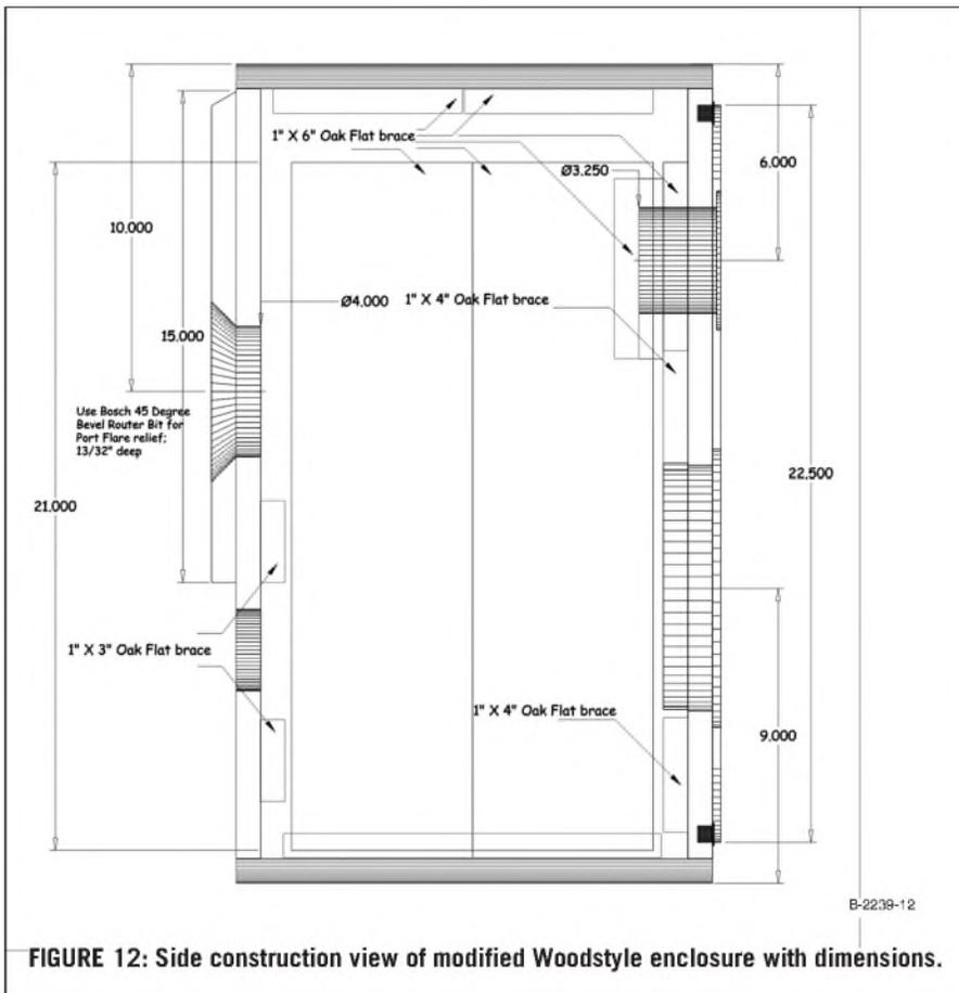
FIGURE 12: Side construction view of modified Woodstyle enclosure with dimensions.
