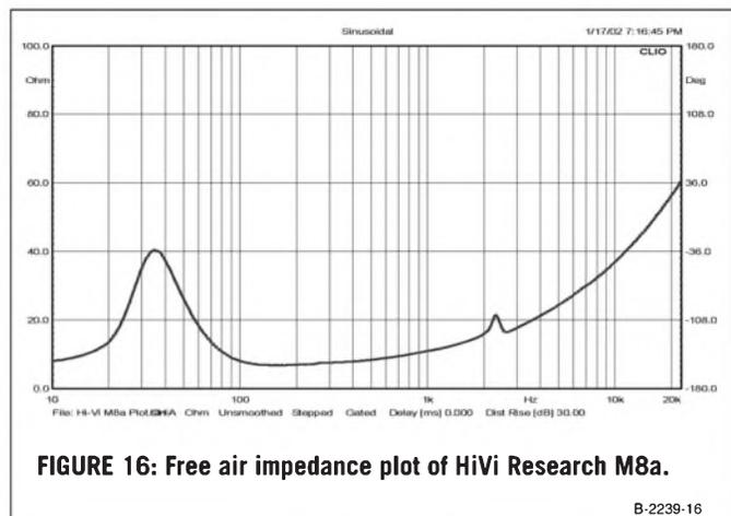
FIGURE 16: Free air impedance plot of HiVi Research M8a.
