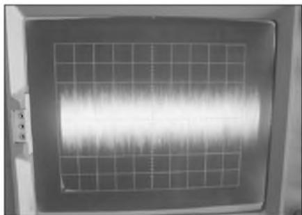
PHOTO 7: Galo supply noise scope (100µV/div RTI, 2ms/div, 42µV RMS).
