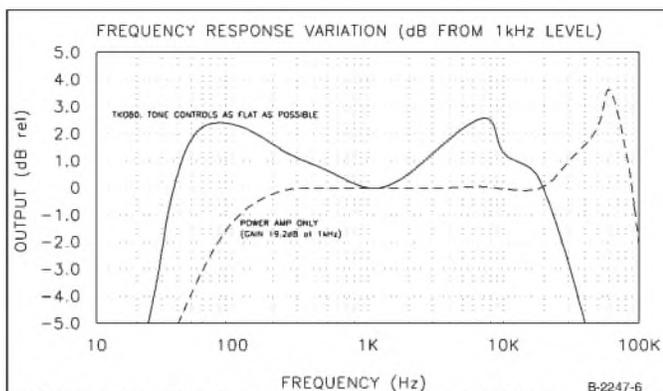
FIGURE 6: Amplifier frequency response, stock TKO 80.
