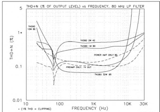
FIGURE 3: THD+N versus frequency, stock TKO 80. B-2247-3
