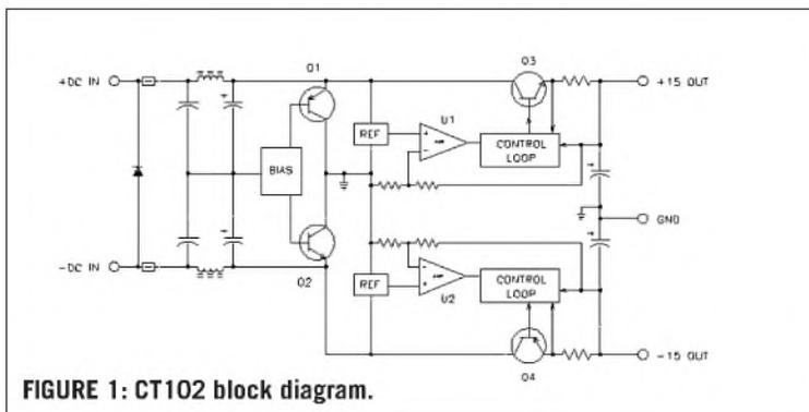
FIGURE 1: CT102 block diagram.
