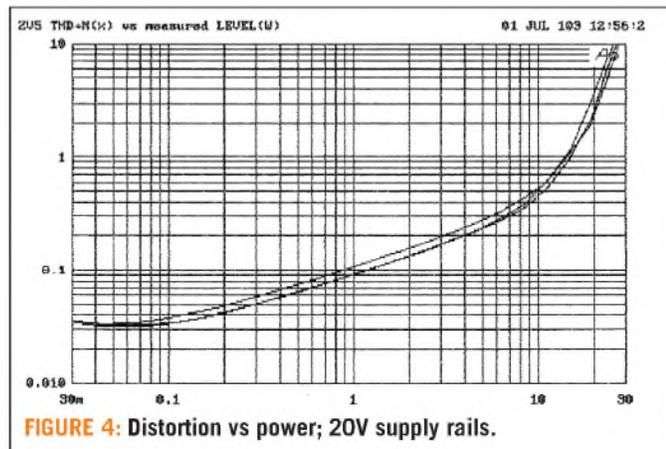
FIGURE 4: Distortion vs power; 20V supply rails.
