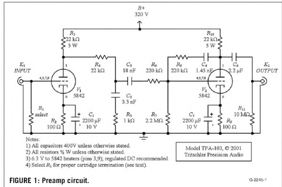
FIGURE 1: Preamp circuit.
