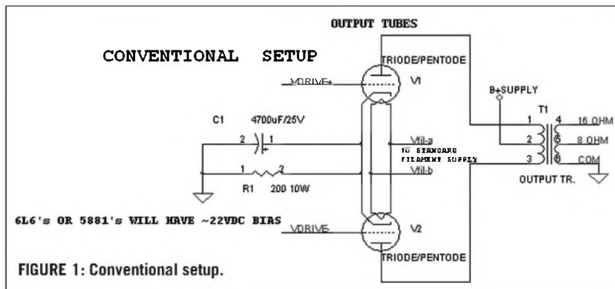
FIGURE 1: Conventional setup.
