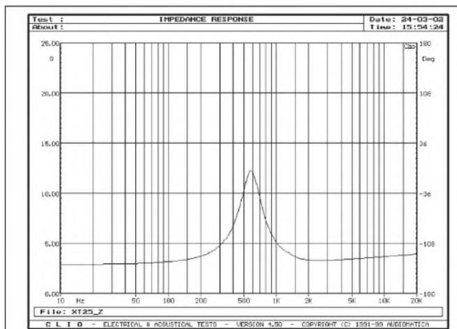
FIGURE 18: Impedance plot for Vifa XT-25.
