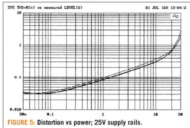
FIGURE 5: Distortion vs power; 25V supply rails.
