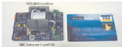
Available as a ready to play audio appliance, or modules for DIY projects. Almost no heat sinking is called for, a thin steel sheet metal floor of the enclosure will do! Build as mono blocks, stereo, 5 ch, 7 ch in one enclosure. 200 W/8 400W/4 650W/2 RMS cont. pwr. 5 - 150,000 Hz +/- 3dB THD 0.02% @ 10W Damping Factor 130 Max. Current 62 Amp.
