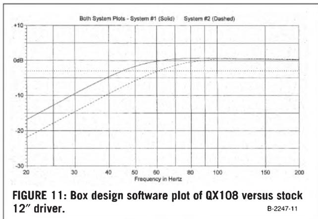
FIGURE 11: Box design software plot of QX108 versus stock 12" driver. B-2247-11
