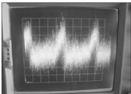
PHOTO 8: LM340/LM320 supply noise scope (100µV/div RTI, 2ms/div, 105µV RMS).
