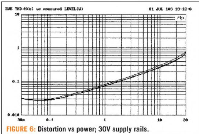
FIGURE 6: Distortion vs power; 30V supply rails.
