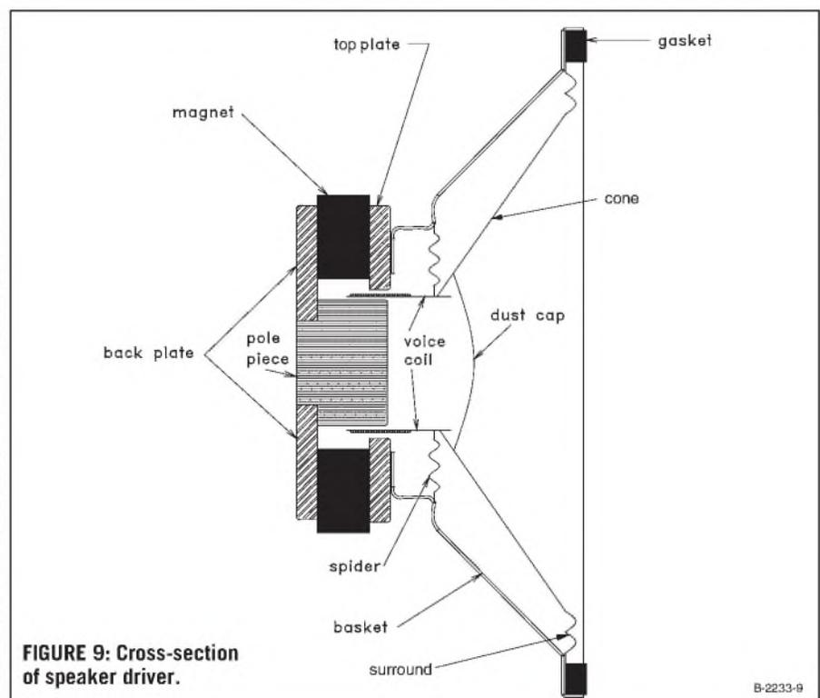
FIGURE 9: Cross-section of speaker driver.
