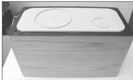
**PHOTO 6:** Driver recesses routed in front panel build-up.
