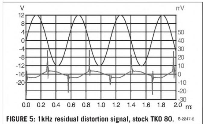
FIGURE 5: 1kHz residual distortion signal, stock TKO 80.
