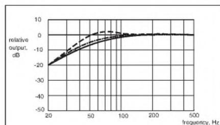
FIGURE 13: Frequency responses for sealed cabinets of different sizes.
