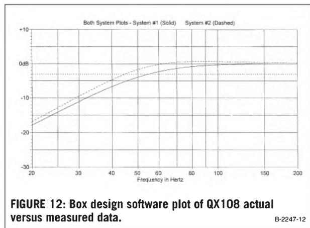
**FIGURE 12: Box design software plot of QX108 actual versus measured data.**
