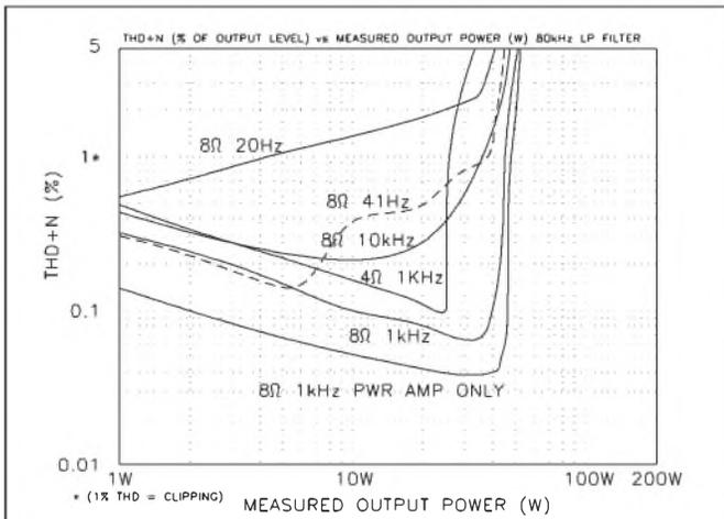
FIGURE 2: THD+N versus output power, stock TKO 80. B-2247-2
