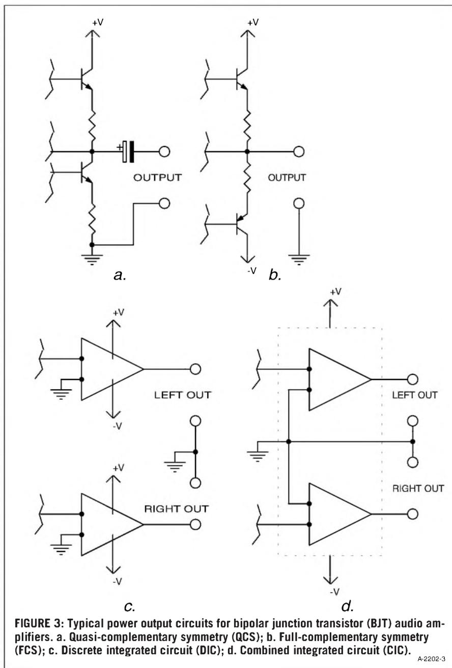
**FIGURE 3:** Typical power output circuits for bipolar junction transistor (BJT) audio amplifiers. a. Quasi-complementary symmetry (QCS); b. Full-complementary symmetry (FCS); c. Discrete integrated circuit (DIC); d. Combined integrated circuit (CIC).
