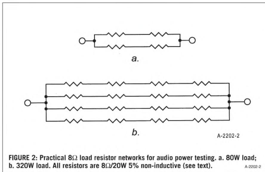
FIGURE 2: Practical  $8\Omega$  load resistor networks for audio power testing. a. 80W load; b. 320W load. All resistors are  $8\Omega/20W$  5% non-inductive (see text).
