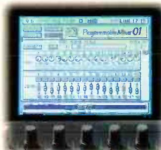
**Remote Control:** Use O2R faders and keys to control outboard mixers, effects, sound modules and transports via MIDI.
