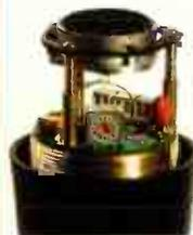
A 16-step variable attenuator and wide range input limiter prevent distortion during extremely high SPL levels. A resonance tuned suspension isolates the cardioid electret capsule to minimize handling noise.
