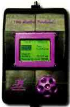
RTA, SPL, ETC. MIDI data monitor, SMPTE read/gen, dB meter, signal generator, S/N, cable tester, phantom power checker, guitar tuner... and a lot more for
