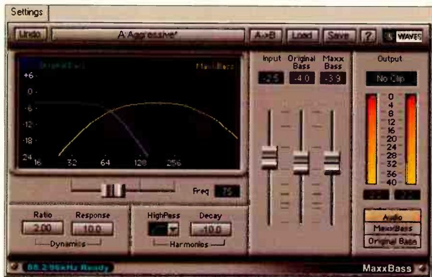
Fig. 1. Waves' MaxxBass isolates the signal's original bass and generates harmonics from it. You can then adjust the blend of the original bass with the bass contributed by the MaxxBass.
