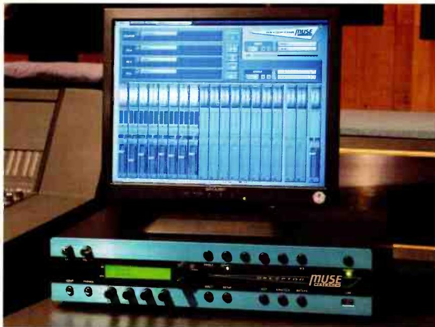
load a VST soft synth/sampler. Each channel can load three VST insert effects (which can be arranged in any series/parallel routing), and there are two effects busses and a master bus with three insert effects each.
