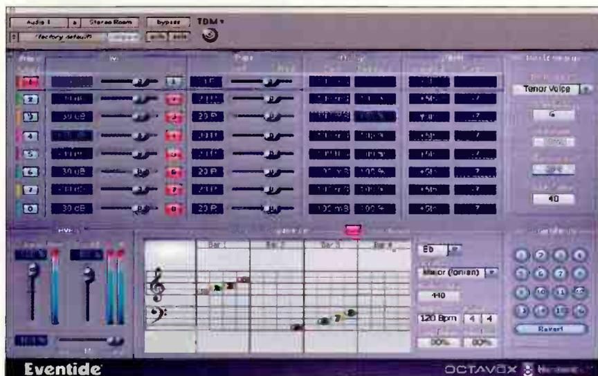
delay times. A snapshot feature provides a way to capture and recall parameter settings with a single mouse-click, and instrument presets optimize Octavox for the pitch recognition characteristics required for various input signals.
