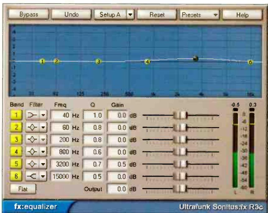
**Fig. 3.** Some equalizers let you adjust the graph's vertical resolution, making it easier to see tiny amounts of EQ. Here, a very broad  $0.5$  dB boost has been added at  $3.2$  kHz.
