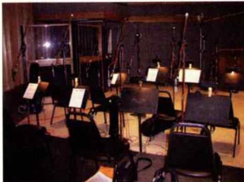
A forest of R-121s and R-122s set up for four trumpets and four trombones. Photo: Royer Labs.
