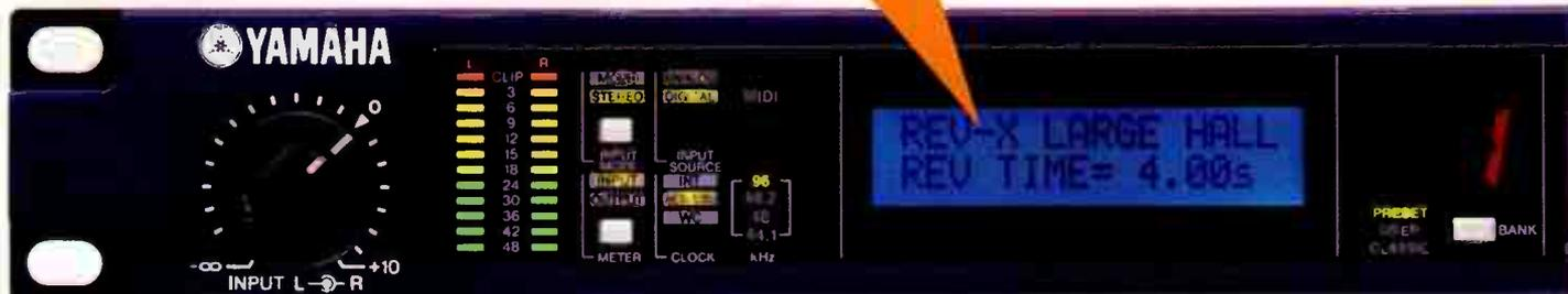
THE SPX2000'S FRONT PANEL FEATURES A VERY EASY TO USE, UNCLUTTERED INTERFACE.
