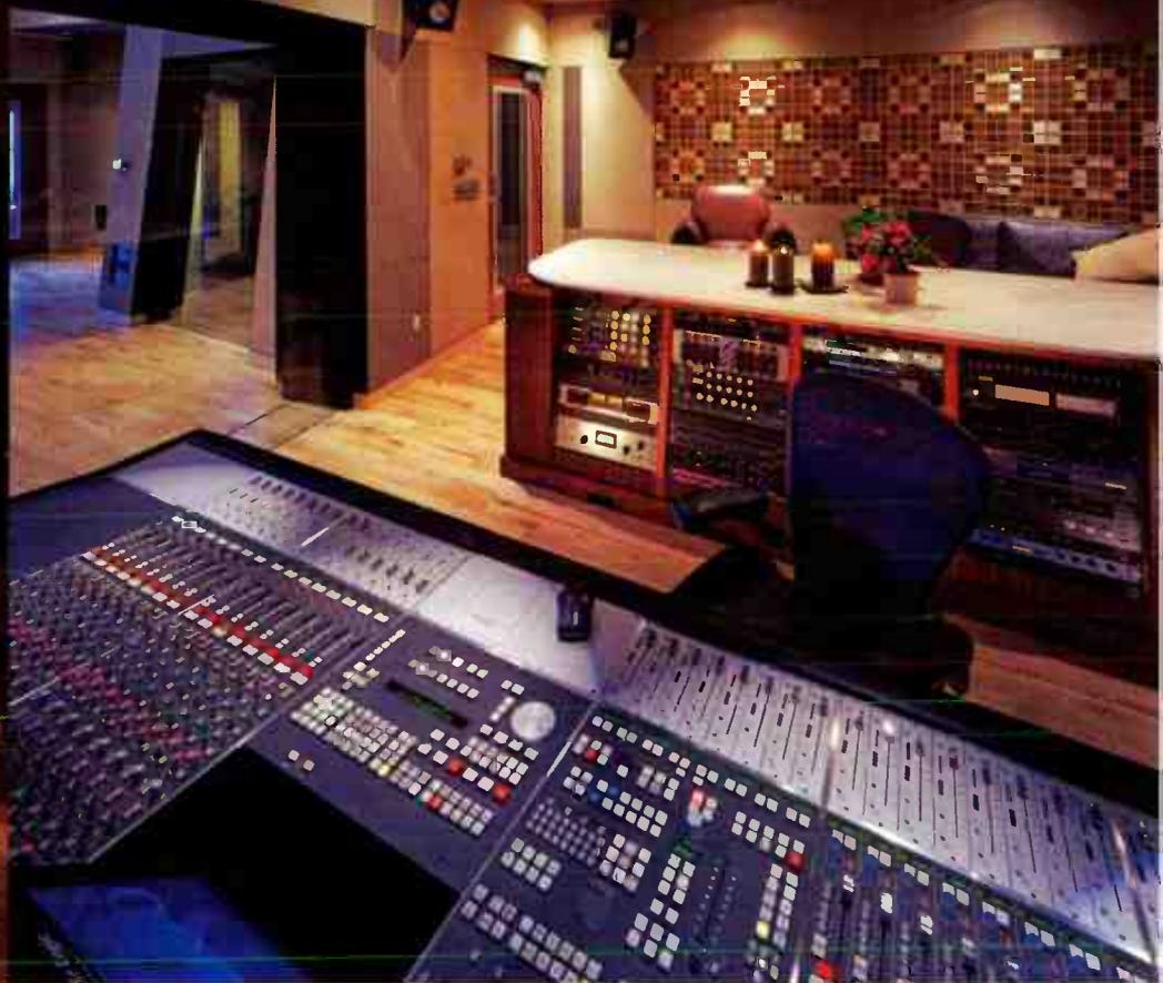
The control room at BiCoastal Music is centered around an SSL C200 console; the studio operates mainly in the digital domain, although a nice selection of outboard gear provides plenty of processing options.
