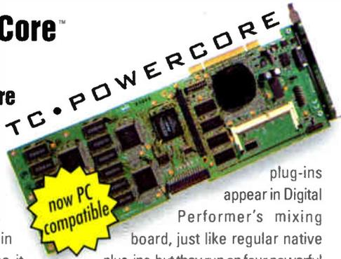
TC•PowerCore is a major breakthrough for Digital Performer's real-time MAS plug-in environment because it provides DSP turbocharged plug-in processing. At last, the renowned TC TOOLS/96 studio-quality FX package (included), with TC MEGAVERB, TC Chorus/DELAY and TC EQ<sup>SP</sup>, can be at your fingertips in Digital Performer, plus other TC | Works
