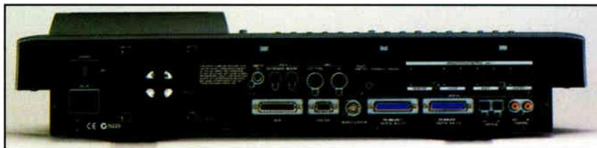
Rear panel I/Os include two R-BUS connectors, Roland's proprietary multichannel digital I/O bus, carrying up to eight channels of 24/96 audio on DB-25 connectors.
