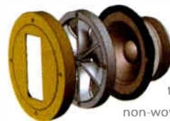
The cone of the all-new 6 in midrange driver created for the KF300z uses a non-woven carbon material to eliminate the distortion associated with the directional bias of a woven material.
