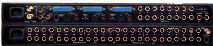
Together, a 2408mk3 and 24i/o give you 32 analog and 24 ADAT/TDIF digital inputs and outputs in a compact, affordable system.
