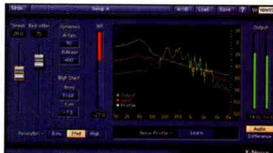
*x-Noise intelligently learns from a section of noise and then applies a broadband noise reduction to eliminate background noise from a source.*
