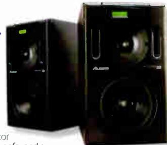
The Alesis ProLinear 720DSP bi-amplified reference monitor has a 7" kevlar woofer and a 1" silk-dome tweeter. It uses a 28-bit digital signal processor to implement the crossover entirely in the digital domain, which also enables you to set and store multiple EQ curves via the built-in 4-band parametric EQ. The PC serial interface allows you to fine-tune EQ settings and control up to 16 speakers remotely. 80 watts LF/40 watts HF amplification. Priced as each
