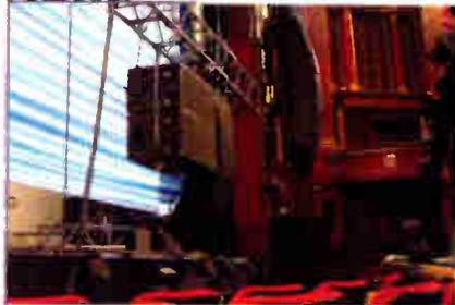
**ABBA tribute musical Mamma Mia! is currently touring Europe with a configuration comprising 10 L-Acoustic KUDOs per side and a center cluster of 11 dV-DOSCs, rounded out by two SB218 subs.**
