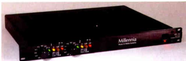
3C (\$1,995) delivers two of the same preamps used in its HV-3D 8-channel units, but in a single rackspace. The transformerless design outputs up to 60.5 dB of gain (78 dB upon request) on a 36-step gain control with both channels gain-matched within 0.8 dB. Options include 130V mic inputs (B&K/DPA), 192kHz/24-bit POW-r A/D converters and DC input. THD+N measures 0.0005%, and gold-plated switches and connectors are used throughout.
