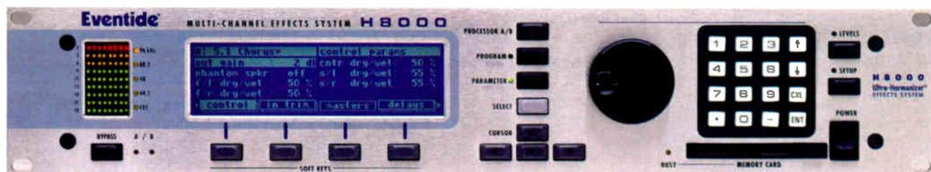
eight AES/EBU, eight ADAT, two S/PDIF and two balanced analog (20 ins and outs total). The analog ins are on XLR/TRS combo jacks, while analog outs are on XLRs; all AD/DAs are 24-bit. All analog I/O can accept unbalanced lines if the cold (pin 3 or ring) signal is shunted to ground, making the H8000 plug-and-play with instrument inputs. (The H8000 can accommodate both line and instrument levels via its pre-A/D boost/cut capability.
