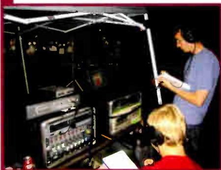
The recording gear included a laptop running Pro Tools through a modified Digidesign 002 Rack.
