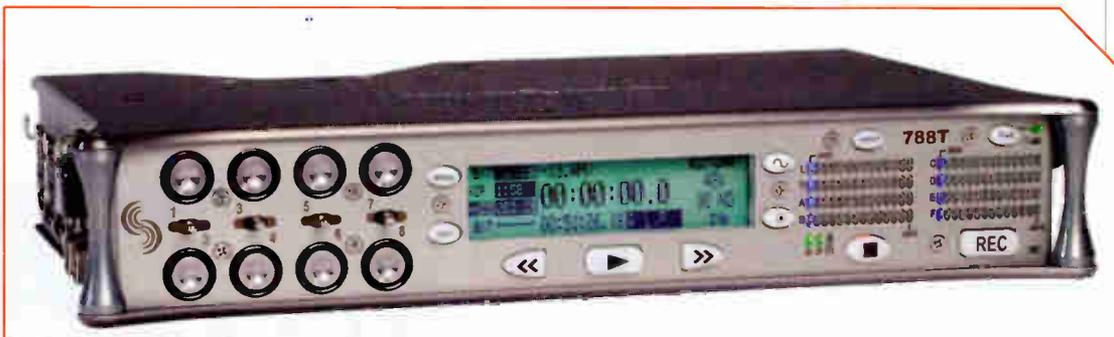
The 788T's front panel features 112-segment (8x14-inch) sunlight-viewable meters, gain control and a backlit LCD screen offering a variety of system information.
