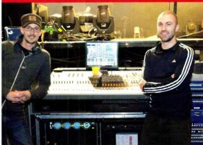
A 96-channel Avid VENUE is seen at monitor world, where engineer Simon Kemp relies on Smack compressors on all vocals—and that's it. "Some additional rack gear I'm using is Dolby Lake EQ on the side-fills," Kemp adds. "I like to keep it very simple; I won't just use something for the sake of it. Less is more in this game. The EQ and dynamics on the desk are very good anyway."
