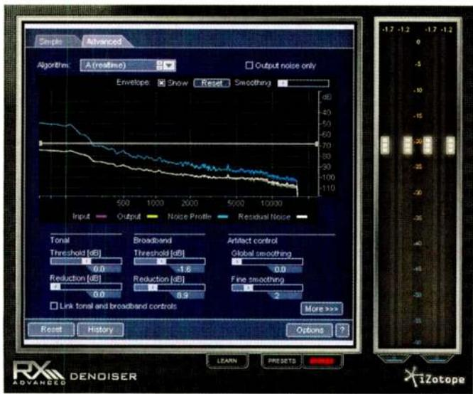
Figure 2: The Denoiser plug-in allows independent attenuation of tonal and broadband noise components.
