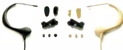
The BP893 MicroEarset combines an ergonomically molded earpiece and omni condenser capsule on a 1-inch boom that fits over either ear. A 55-inch cable connects the mic to an XLR power module (with settings for flat response or 80Hz filter) or directly to an Audio-Technica UniPak bodypack transmitter; terminations for other makers' systems are also offered. Retail is \$479 (in black or beige), including a cable clip, two windscreens, moisture guard and carry case. NAMM booth #6740.
