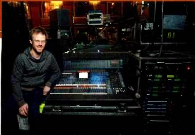
Monitor engineer Colin Burrell mans a Yamaha DM2000, using external A8R preamp/A/D converters for extra inputs into the board, and Aviom A16R and Squirrel Labs Defibrillator. "The band is on in-ears, with no wedges or sidefills," Burrell says. "We're using a Sennheiser IEM system that is great-sounding and very reliable. Some of the band is on ACS ears; others are on Ultimate Ears. I stuck with which models they were using when I started as everyone was happy already."
