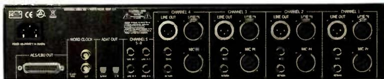
The back panel offers XLR mic in, line in and out, and balanced insert sent/returns on TRS plugs, as well as four extra TRS inputs for the extra line inputs.
