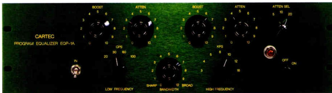
*The EQP-1A features point-to-point wiring and custom-made transformers.*
