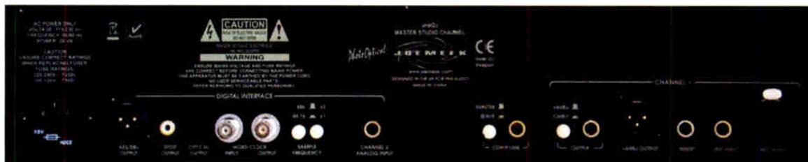
Digital I/O on the unit is impressive with Optical, SPDIF, AES/EBU, and Word Clock I/O.
