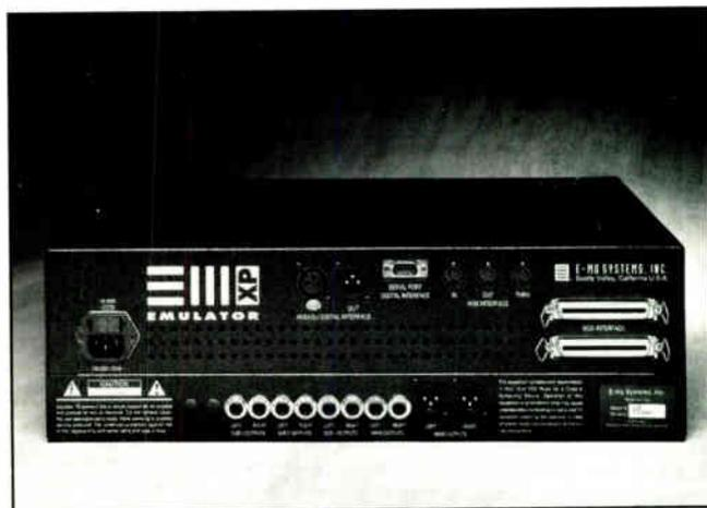
while the 18-bit D/A converter exits through balanced XLR connectors (pin 3 hot—groan!) and balanced 1/2-inch phone jacks. The stereo submix outputs are a good addition for professionals, with each channel having its own TRS (balanced) output—no
