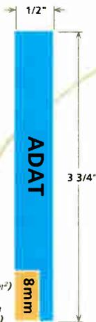
Comparison of tape areas for 1 second of audio: ADAT (1.211 mm<sup>2</sup>) and the 8 track, 8mm helical scan format (133 mm<sup>2</sup>).
