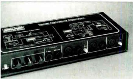
units in the chain. This offers each performer control of a personal mix, while leaving the monitor/cue mix unchanged. Multi-Send has selectable mono and stereo modes with balanced or unbalanced operation, along with two headphone outputs and a 1/4-inch line level out for feeding stage monitors. Retail is \$349.
