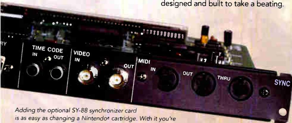
Adding the optional SY-88 synchronizer card is as easy as changing a Nintendo® cartridge. With it you're SMPTE and MIDI compatible. And no matter how many DA-88s you have locked up, you need only one sync card. Other optional accessories include AES/EBU and SDF2 digital interfaces allowing the digital audio signal to be converted for direct-digital interfacing with digital consoles, signal processors and recording equipment.
