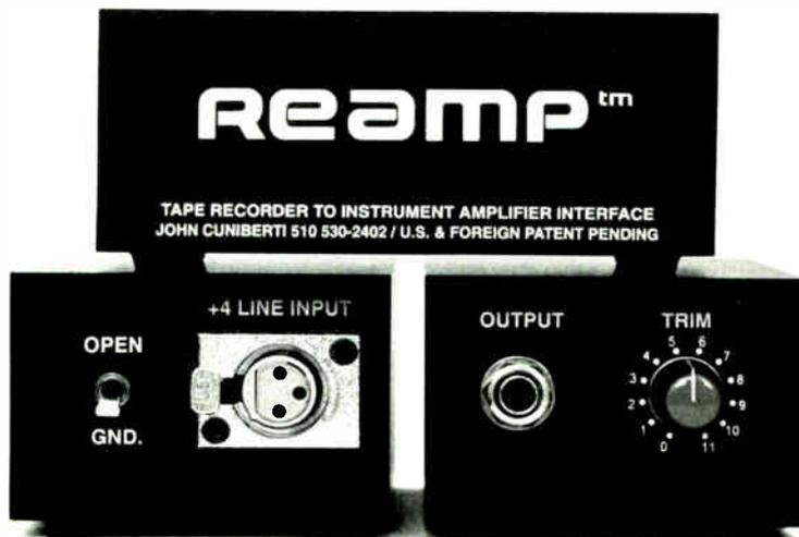
REAMP is about the size and shape of the popular Countryman direct box. Because it is passive, there are no batteries to change, and it is RF-protected. On the input side is a ground lift switch and a female XLR +4dBu connector in which to plug your tape track output. On the output side is a volume trim pot (yes, it goes up to 11) and a 1/2-inch jack for connection to an amp.
