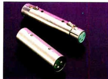
Switchcraft® offers a complete line of adapters including the 3-contact female to female, #389 (with Switchcraft A3F inserts at both ends) and the 3-pin male, #390 (with Switchcraft A3M inserts at both ends). Both the #389 (shown at top of photo) and the #390 (shown at bottom of photo) have pre-wired contacts. The female version has a polarizing boss; the male version has a polarizing groove.
