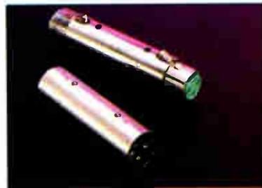
Switchcraft® offers a complete line of adapters including the 3-contact female to female, #389 (with Switchcraft A3F inserts at both ends) and the 3-pin male, #390 (with Switchcraft A3M inserts at both ends). Both the #389 (shown at top of photo) and the #390 (shown at bottom of photo) have pre-wired contacts. The female version has a polarizing boss; the male version has a polarizing groove.
