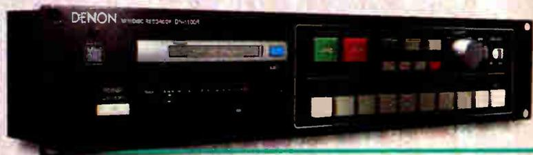
**DN-1100R MD Recorder** The DN-1100R MD recorder offers 74 minutes of stereo recording time with a 44.1 kHz sampling rate, 16-bit linear (A/D converter) quantization and ATRAC compression. The unit also features 10 independent "Hot Start" buttons to which any 10 tracks from a total of 255 can be assigned. This feature is ideal for sound effects libraries, sound bytes and announcements.
