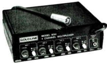
Automatically samples information from 4 microphones in a single test and captures the overall room response across the entire seating area.
