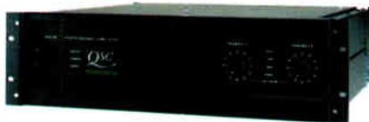
**THE POWERLIGHT™ 4.0, WHICH DELIVERS 2000 W/CH. AT 2Ω, FEATURES SEVERAL NEW IMPROVEMENTS INCLUDING CLIP LIMITERS AND A DATA PORT CONNECTOR INTERFACE TO QSC'S MULTISIGNAL PROCESSOR (MSP) PROVIDING DIGITAL SIGNAL PROCESSING AND CONTROL AND MONITORING BY COMPUTER OVER AN ETHERNET NETWORK.**
