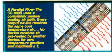
Books have been written about thermal management, but it all boils down to three things: air flow, heat sink area, and  $\Delta T$  (the difference between the heat radiator and ambient air). The CS 800S uses a unique "parallel flow" heat sink alignment so every transistor receives the same cool temperature air for optimum  $\Delta T$ .
