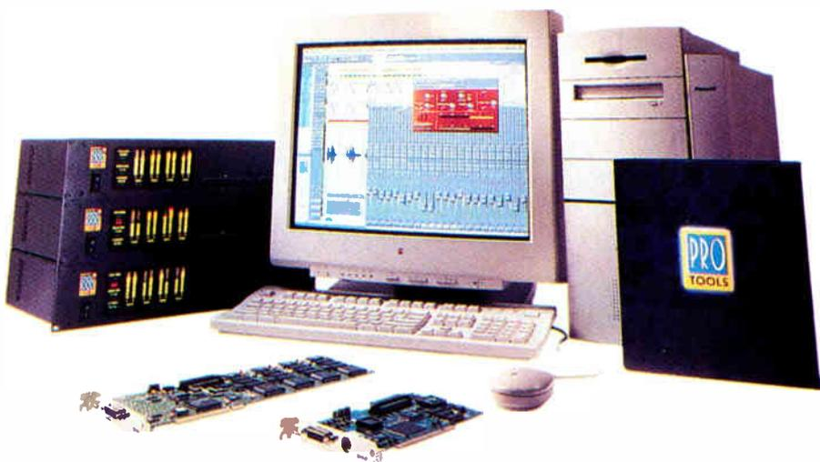
of this writing) software. The d24 card is capable of recording and playing up to 32 tracks of 24-bit or 16-bit audio, provided that the hard disk and SCSI bus are fast enough.
