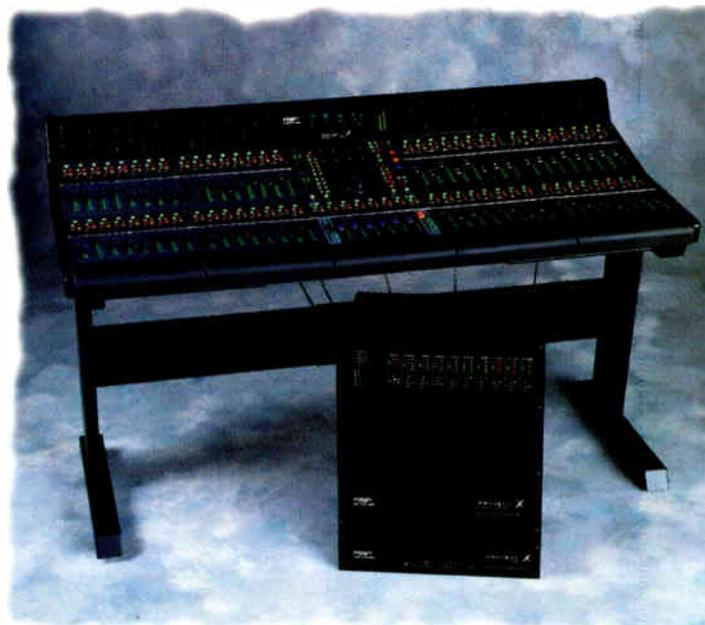
Project X is available as a 32 channel system, expandable to 48 or 64 input channels with 8, 16, or 24 simultaneous track assign buses. Upgradable software. Applications include music mixing, audio post, mix to pic productions and sound design. Made in the USA.
