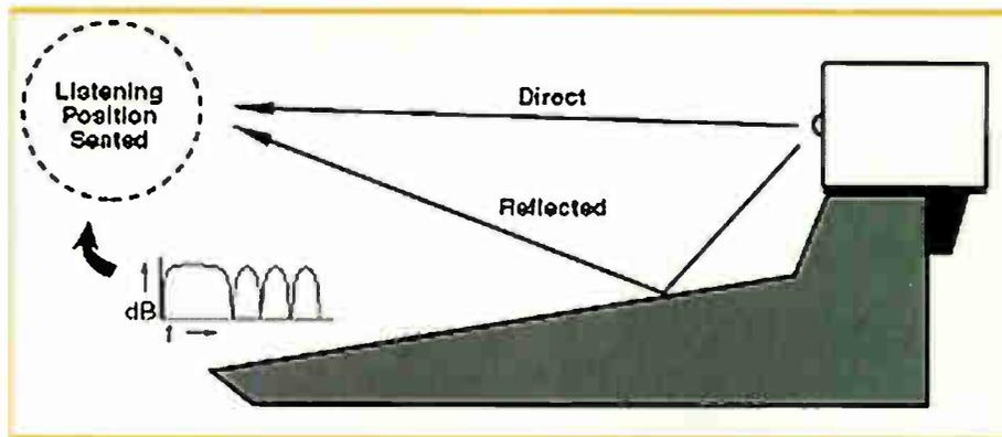
Figure 5: Reflections interact with listener (causing comb filtering) when speaker is placed on console top.
