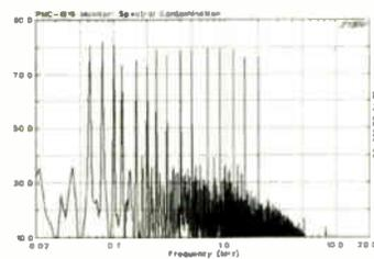
Spectral contortion distortion is around 40 to 45 dB below the input test tones in the mid band, and improves at lower frequencies.
