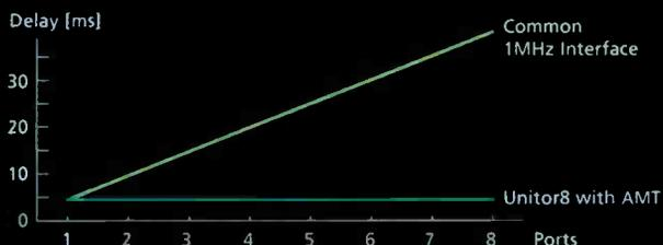
Thanks to the AMT technology (Advanced MIDI Transfer) the Unitor8 is the only 8x8 MIDI interface that is capable of sending data to all ports simultaneously, even with 8 units stacked together.
