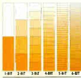
Every bit you add doubles the resolution of a digital recorder. Compared to 16-bit formats, ADAT Type II's non-compressed, linear 20-bit recording offers a wider dynamic range, less quantization distortion at low levels, more headroom and even lower noise. Result: detailed, full-spectrum audio fidelity that far exceeds the quality of any analog recorder.
