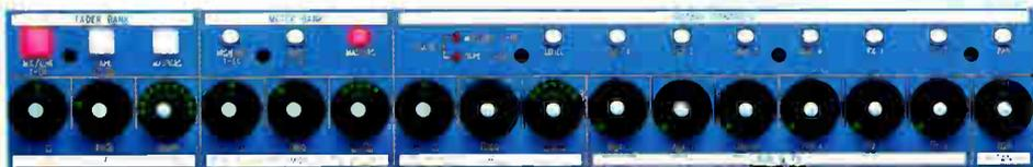
...A HORIZONTAL INPUT CHANNEL WITH FULL EQ, AUX AND PAN FACILITIES...
