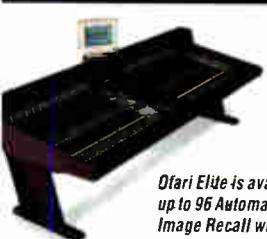
*Otari Elite is available with up to 96 Automated Faders, Image Recall with Snapshot memory and Master Status Switching. Film and Post Production multi-format panning versions are available.*
