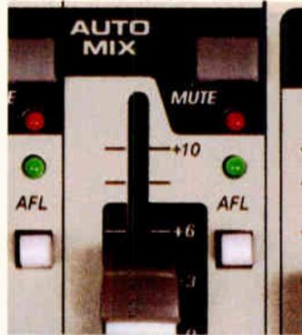
**Automix™** is an 8-channel gain-sharing protocol that tames the comb filtering and phasing issues that occur when multiple microphones compete for dominance in the mix
