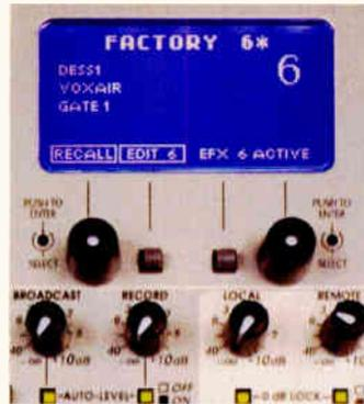
**DSP** section includes a complete rack processing system with Feedback Ferret®, a full digital effects suite, USB connection for streaming audio to a recording interface, designated ambience microphone inputs and broadcast-ready outputs
