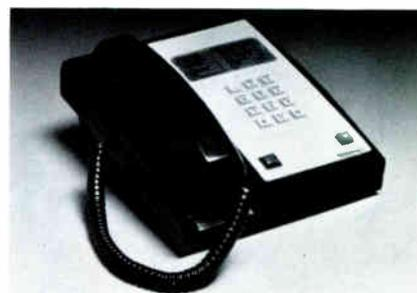
on central offices. All models incorporate the SureTouch dialer which uses integrated circuits in place of electromechanical parts. One model is a single-line telephone with optional transfer access key and optional message waiting lamp; it is intended for PBX applications.
