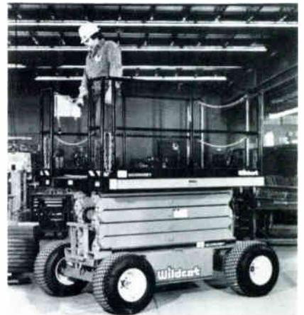
A 24-hour self-timing charger is built in, as are fork-lift pockets at both ends. Working heights up to 32 feet, and capacities to 1000 pounds may be specified.
