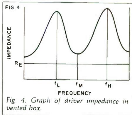
Fig. 4. Graph of driver impedance in vented box.
