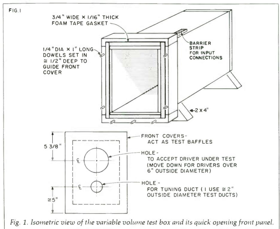
Fig. 1. Isometric view of the variable volume test box and its quick opening front panel.
