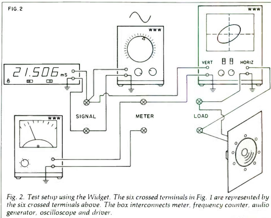
Fig. 2. Test setup using the Widget. The six crossed terminals in Fig. 1 are represented by the six crossed terminals above. The box interconnects meter, frequency counter, audio generator, oscilloscope and driver.
