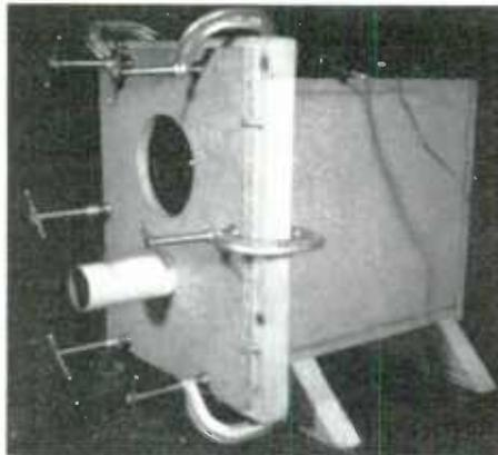
Fig. 3B. Front and side view of box. Note that the tube port is mounted outside so that it does not affect enclosure net volume.
