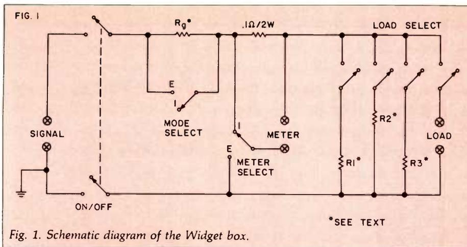
Fig. 1. Schematic diagram of the Widget box.
