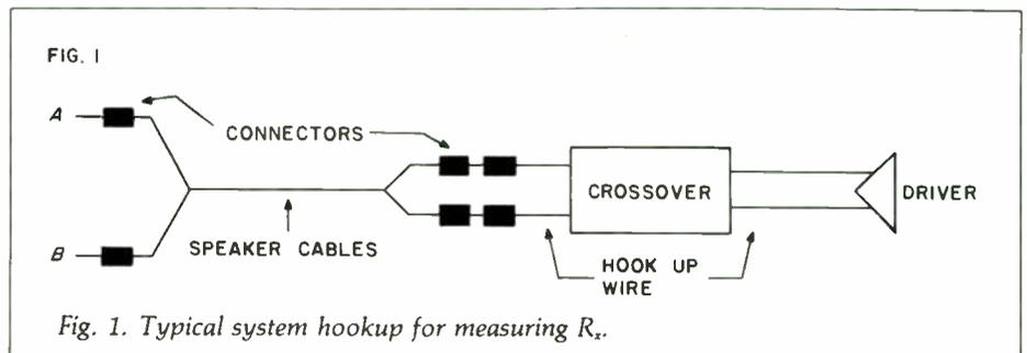
Fig. 1. Typical system hookup for measuring  $R_X$ .
