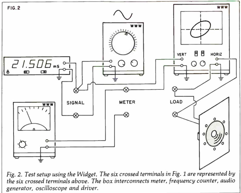
Fig. 2. Test setup using the Widget. The six crossed terminals in Fig. 1 are represented by the six crossed terminals above. The box interconnects meter, frequency counter, audio generator, oscilloscope and driver.
