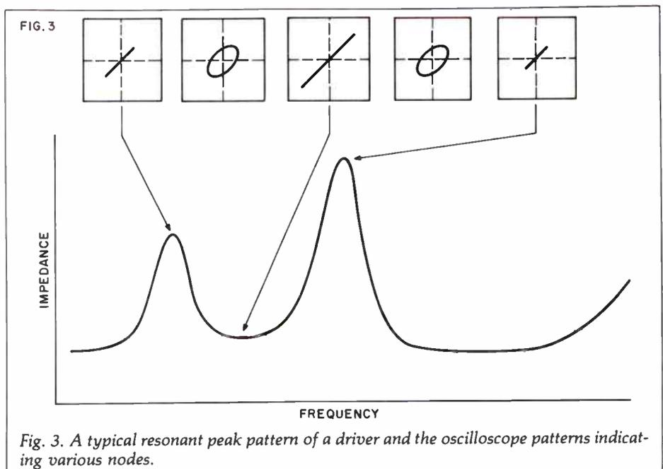
Fig. 3. A typical resonant peak pattern of a driver and the oscilloscope patterns indicating various nodes.
