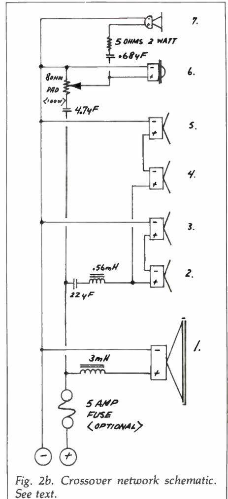
Fig. 2b. Crossover network schematic. See text.
