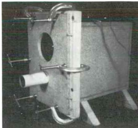
Fig. 3B. Front and side view of box. Note that the tube port is mounted outside so that it does not affect enclosure net volume.
