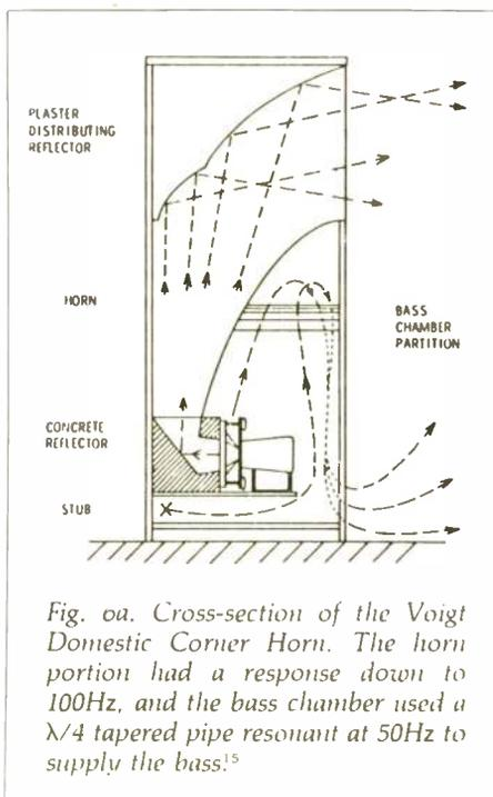
Fig. 0a. Cross-section of the Voigt Domestic Corner Horn. The horn portion had a response down to 100Hz, and the bass chamber used a  $\lambda/4$  tapered pipe resonant at 50Hz to supply the bass.<sup>15</sup>
