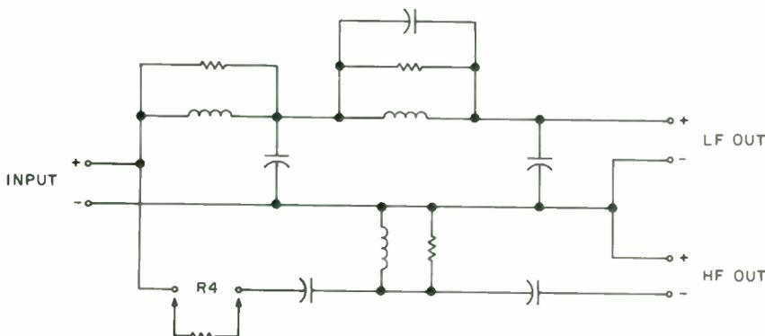
Fig. 5. Crossover network schematic. See text for values, which are proprietary to the kit designer, but are also very difficult to duplicate accurately by traditional value designations.
