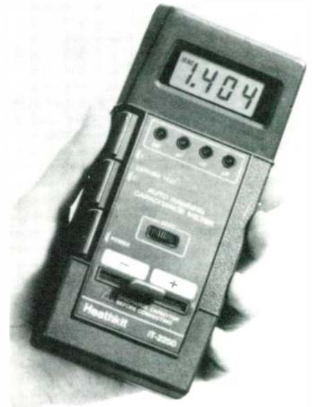
**Heath** is now offering a hand held capacitance meter with a range of .1pF to 199.9uF. The 1T-2250 kit, priced at \$157.95, has a 3 $\frac{1}{2}$  digit display, auto ranging, and a way of measuring directly at cap leads to lessen error. Low voltage measures of small caps are possible as well. A battery eliminator is available for the unit also. Information from **Heath** at Benton Harbor, MI 49022, of course.
