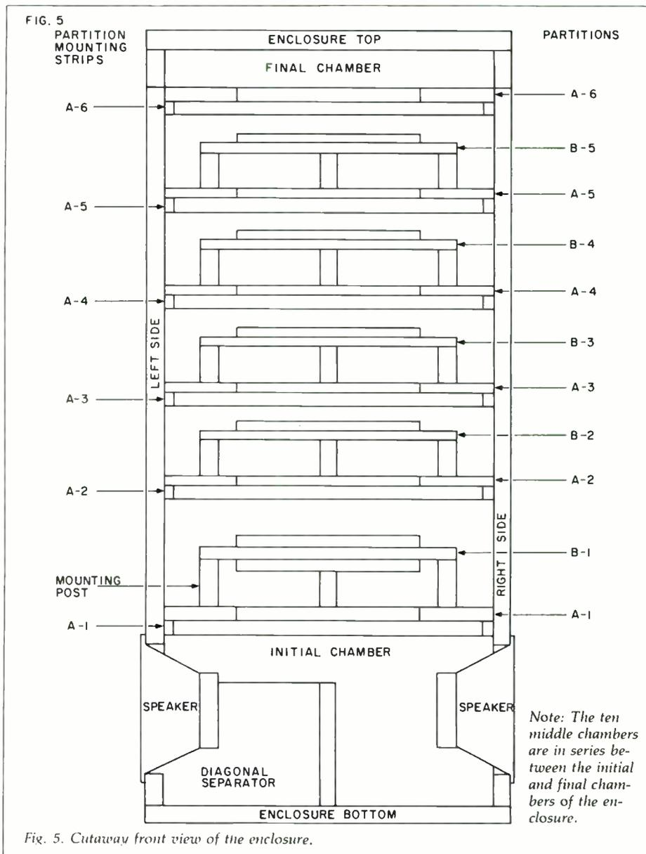
Fig. 5. Cutaway front view of the enclosure.
