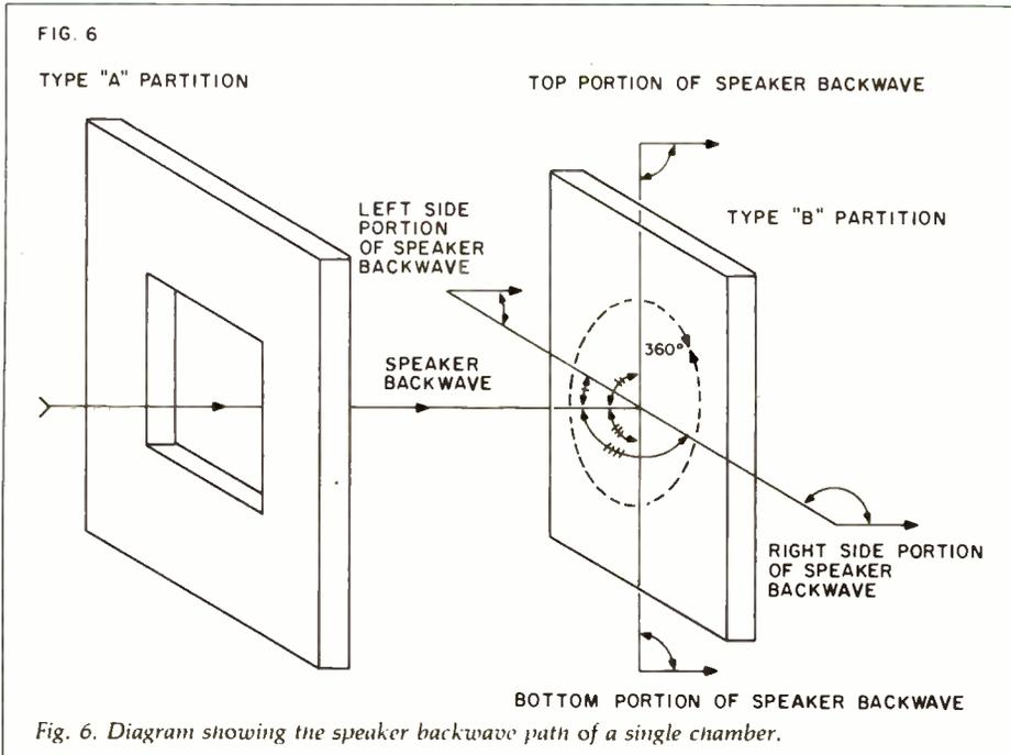
Fig. 6. Diagram showing the speaker backwave path of a single chamber.
