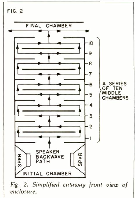
Fig. 2. Simplified cutaway front view of enclosure.
