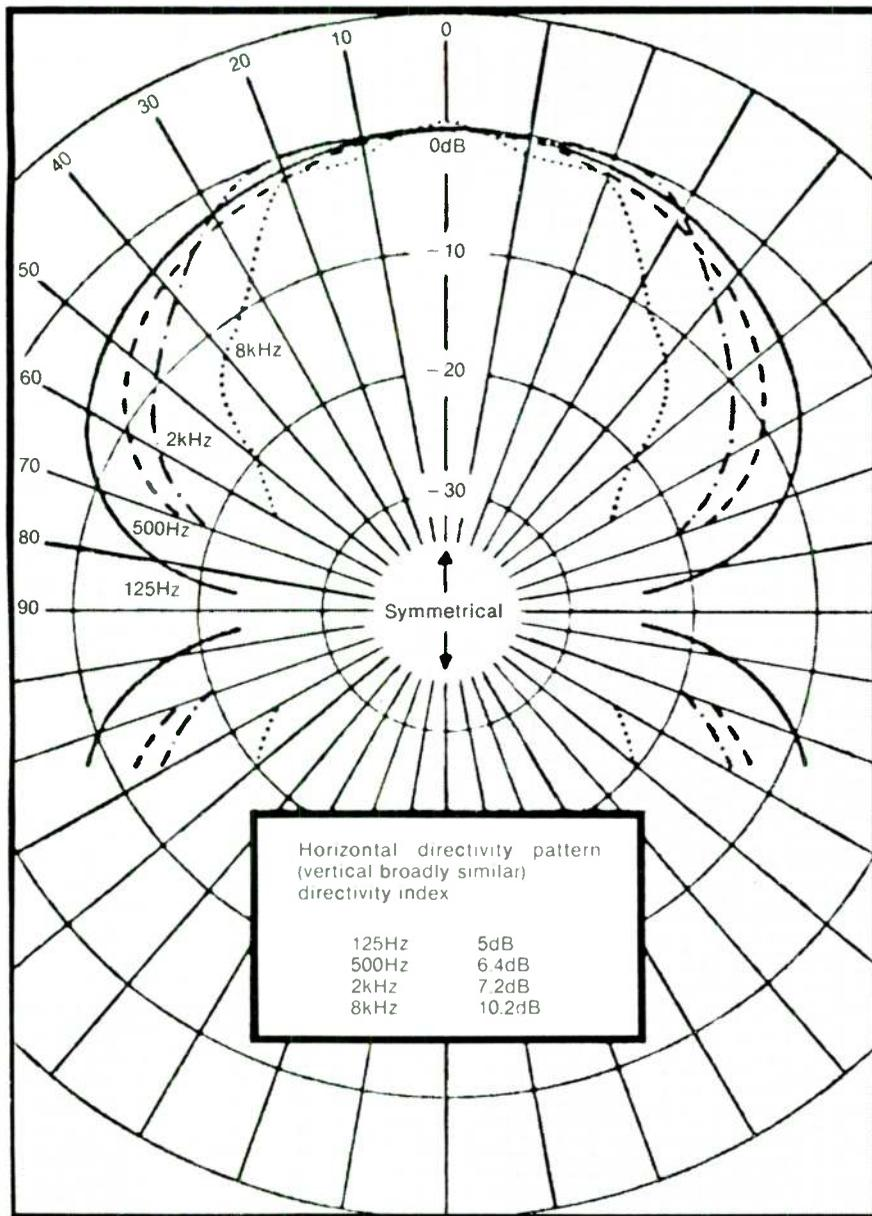
Fig. 7. Measured radiation patterns of the ESL-63.
