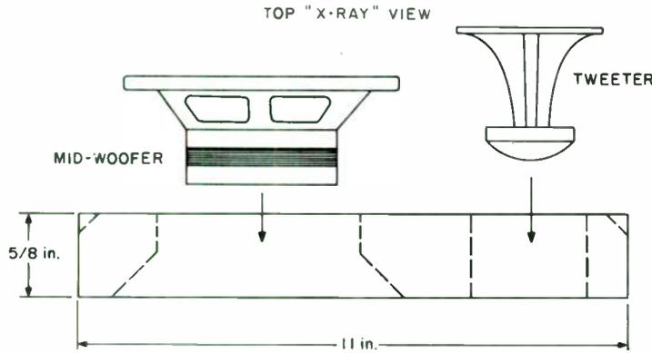
Fig. 3. Cutting details for the acrylic panel.
