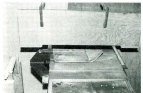
Fig. 6. Table saw setup for cutting large pieces of plywood or particle board.
