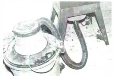
Fig. 8. Vacuum attachment for the table saw.
