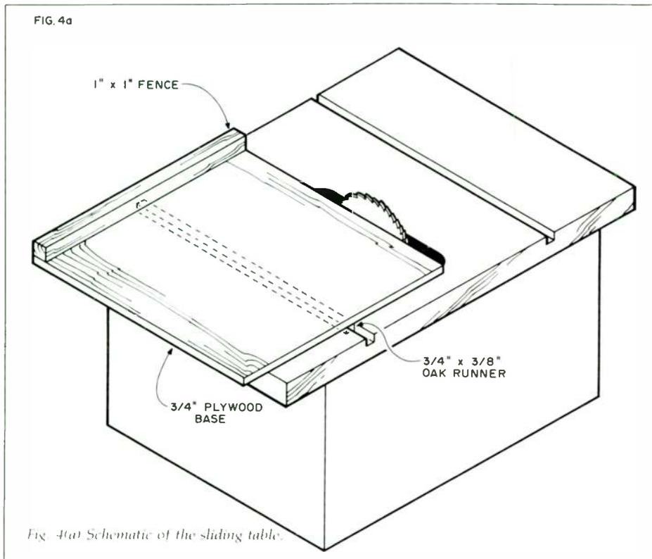
Fig. 4(a) Schematic of the sliding table.
