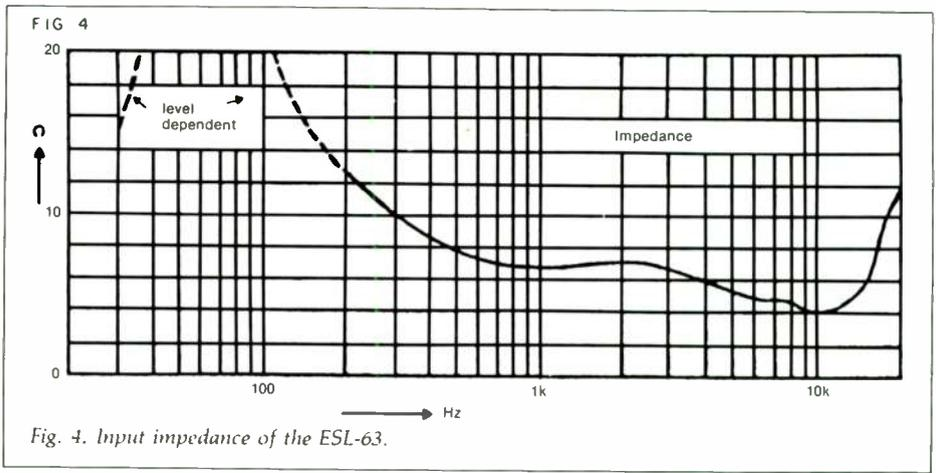
Fig. 4. Input impedance of the ESL-63.
