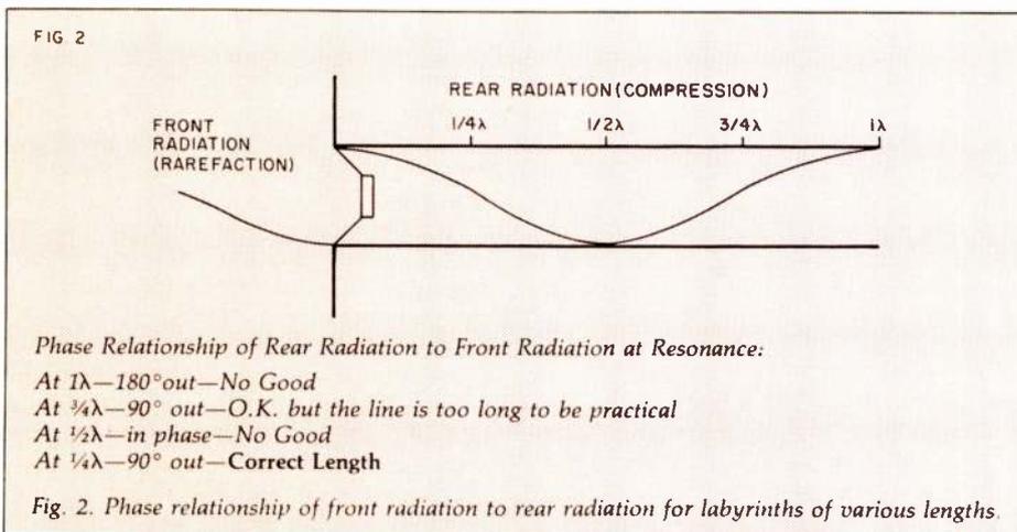
Fig. 2. Phase relationship of front radiation to rear radiation for labyrinths of various lengths.
