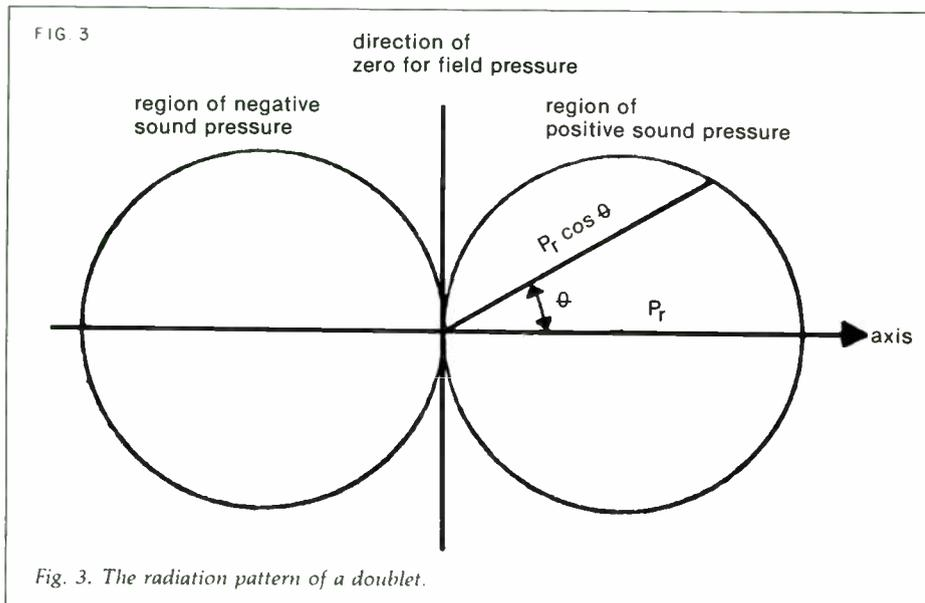
Fig. 3. The radiation pattern of a doublet.
