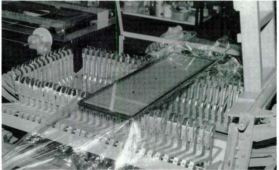
Fig. 12. One diaphragm sits atop the custom made jig which stretches the film evenly over the frame before being bonded to it.
