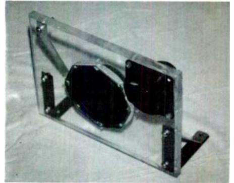
Fig. 4. Front view of the acrylic mid-woofer board.
