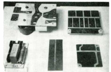
FIG. 1. A group of knife-cut circuit boards.
