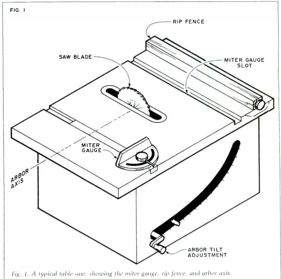
Fig. 1. A typical table saw, showing the miter gauge, rip fence, and arbor axis.
