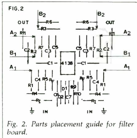
Fig. 2. Parts placement guide for filter board.
