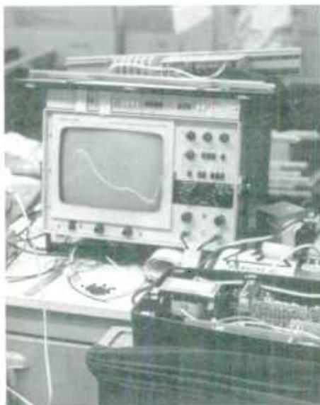
Fig. 16. Testing the ESL-63 for impedance.
