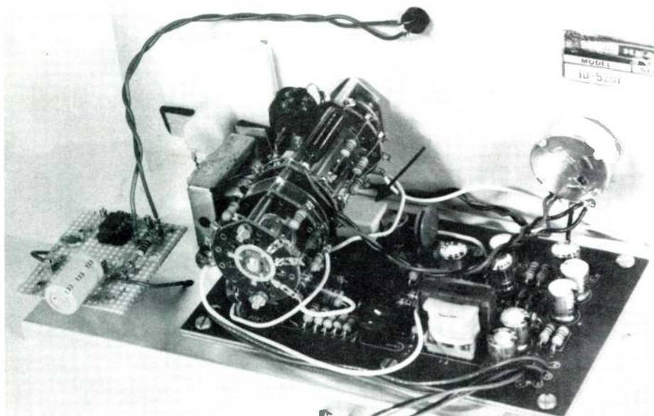
Photo 2. Arrow shows location of new  $C_{10}$  capacitor.
