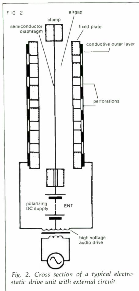
Fig. 2. Cross section of a typical electrostatic drive unit with external circuit.
