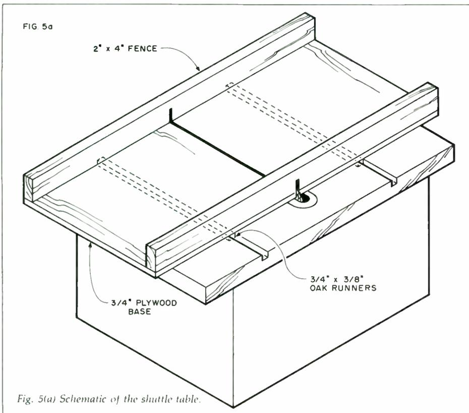
Fig. 5(a) Schematic of the shuttle table.
