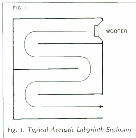
Fig. 1. Typical Acoustic Labyrinth Enclosure
