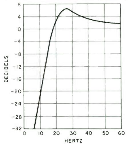
FIGURE 11. Rumble filter has steep rolloff, and the bass boost flattens the woofer's response.
