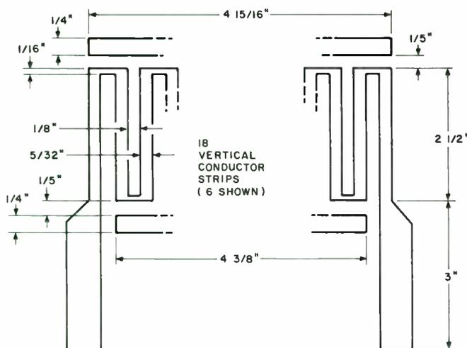
**FIGURE 6:** Use this pattern for the 2:1 conductor.
