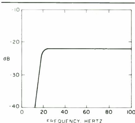
**FIGURE 1:** With the author's WOOF software, the computer plots a theoretical woofer frequency response. This curve is generated from the data listed in Table I.
