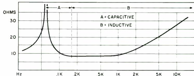
FIGURE 1: A typical woofer has this impedance curve. Unless you compensate for these impedance variations, the frequency response will vary also.
