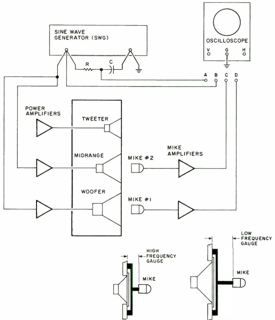
**FIGURE 7.** This test setup measures the phase difference between drivers. After determining which quadrant each is in, use a diagram such as Fig. 9 to help visualize the difference. This will determine actual values for R and C in the phase shifting circuits.
