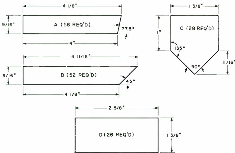
**FIGURE 4:** Have a machine shop cut the magnets' focus plates from 13 gauge steel. Stacks of alternating A and B plates form the two pairs of front focus plates for two Heils. The two sets of rear focus plates use alternating C and D sections.
