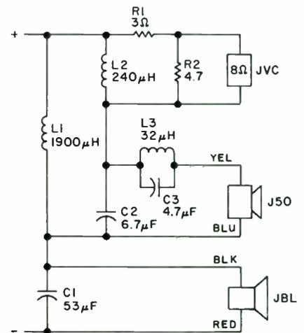
**FIGURE 6:** Although active crossovers are preferable, this simple single-pole three-way crossover works well. L1 & C1 set the 500Hz crossover point, and L2 and C2 set a 4kHz upper crossover. L3/C3 is a 13kHz trap for the J50. This is a six ohm system.
