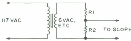
FIGURE 1.  $R_1$ ,  $R_2$  are an optional voltage-divider, if output voltage of xfmr is on the highside.
