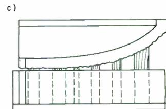
FIGURE 1C: To make fiberglass panels, first make a plaster cast of the contour. The wooden dowels support the wire mesh holding the plaster against the horn contour previously made.
