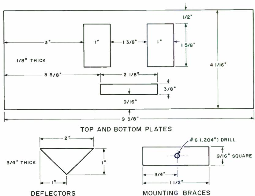
FIGURE 3: Make the Heil driver's top and bottom plates of FRP, masonite, or aluminum.
