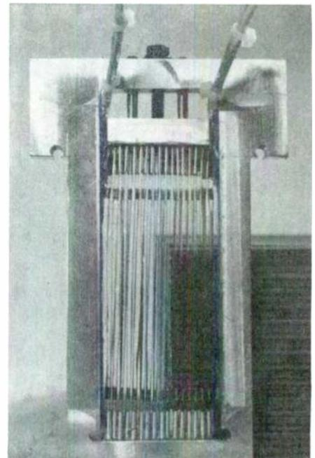
**FIGURE 7:** The diaphragm mounting frame holds the pleated driver. Tension can be adjusted with the nut at the top.
