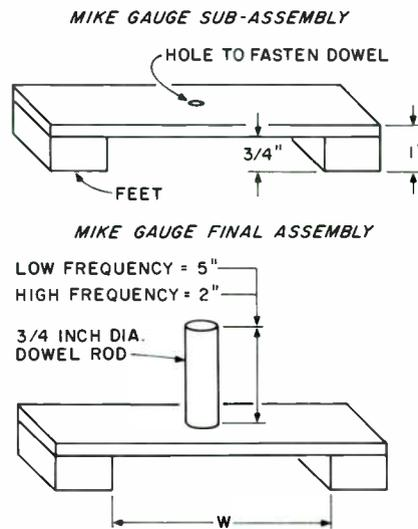
FIGURE 8. Make these gauges very precisely so that accurate measurements result. Keep all reflecting surfaces (including test gear and yourself) well away from the mikes.
