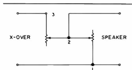
FIGURE 1: Schematic for adjustable L-pad.
