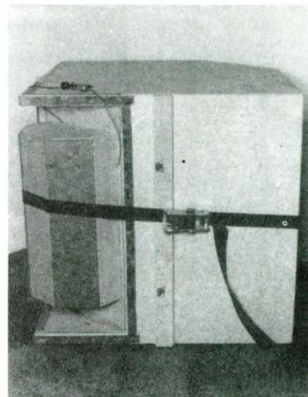
FIGURE 17: Clamp on one of the back chambers to test for system response.
