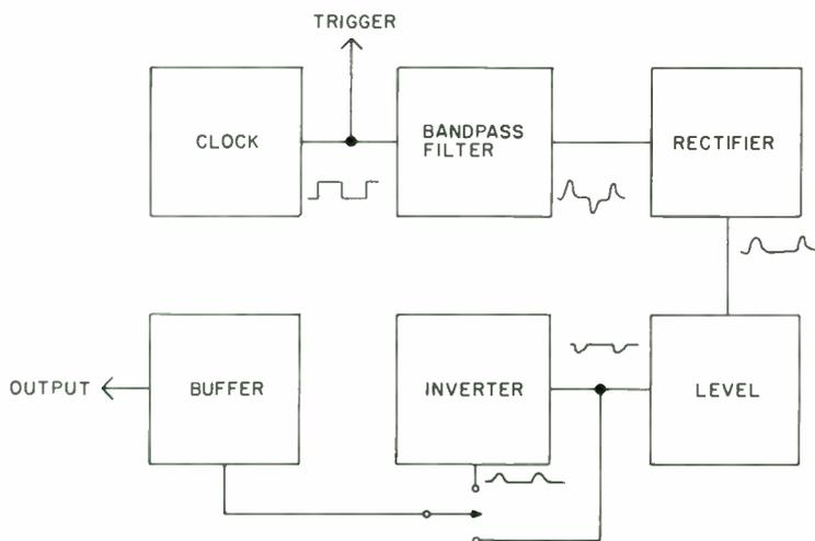
FIGURE 1: The clock generates a simple square wave, which is the trigger for the scope. At the same time, the square wave is shaped by the filter and rectifier into a series of positive-only pulses. At the inverter, a switch enables you to select positive or negative pulse trains.
