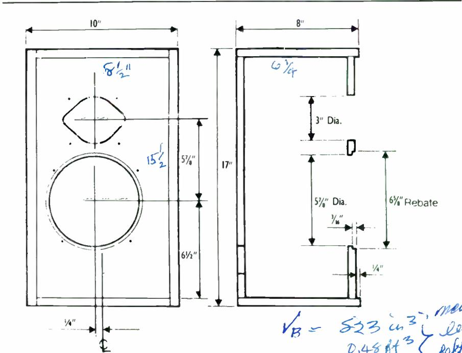
FIGURE 3: Enclosure dimensions for the Timbrel speakers.
