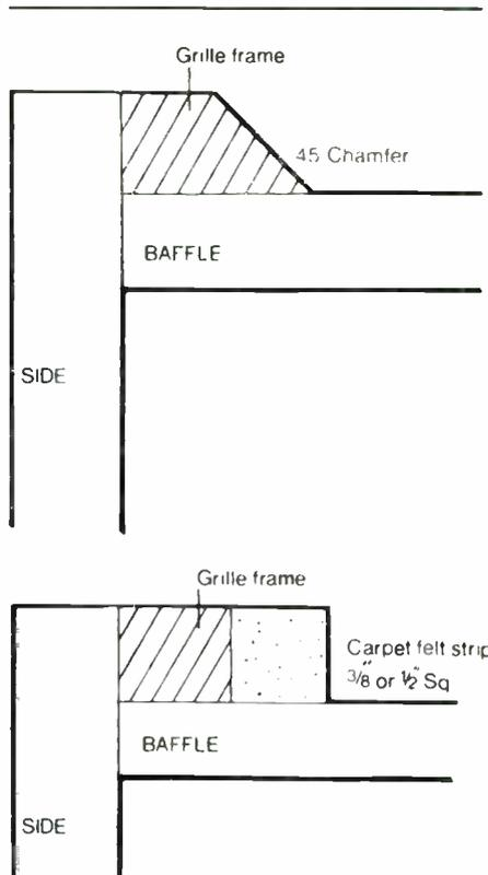
**FIGURE 6: Grille frame construction details show methods of either beveling the inner edge or adding jute rug pad material to diminish diffraction problems.**
