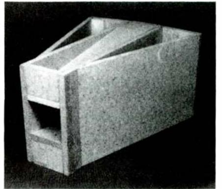
**FIGURE 10:** The folded structure becomes clear at this stage. The throat opening is at the rear.
