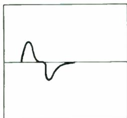
**FIGURE 4:** If the manufacturer has reversed the polarity between the two drivers, the pattern on the scope looks like this.
