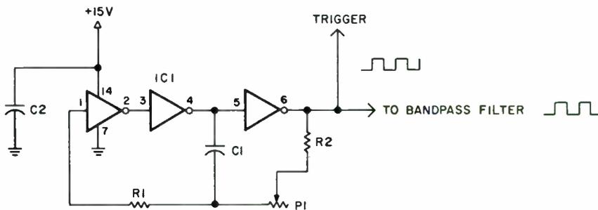
**FIGURE 7:** The schematic for the clock is a square-wave oscillator built from three inverting buffers.
