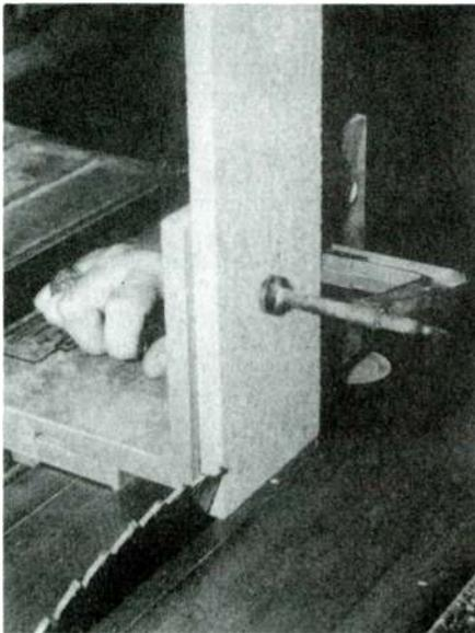
**FIGURE 7:** Use a table saw with a tenon jig to cut the angles easily and safely.
