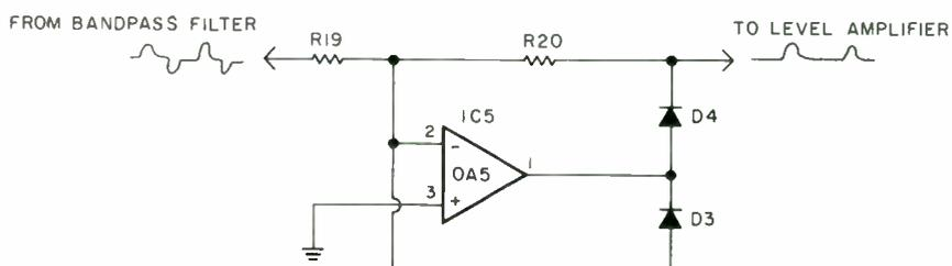
**FIGURE 9:** The rectifier passes only positive pulses.
