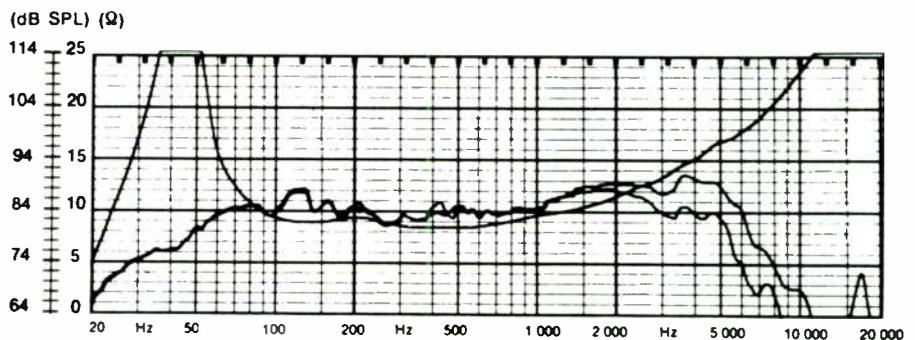
FIGURE 2: The Audax 6 1/2-inch bass/midrange driver (HD17B25H) curves on axis and 30° off axis, plus its impedance curve.
