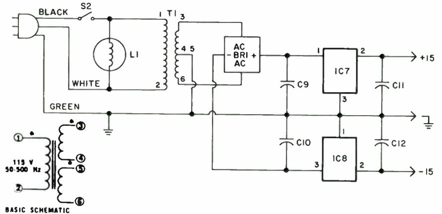
**FIGURE 11:** The power supply is a full wave bridge rectifier.
