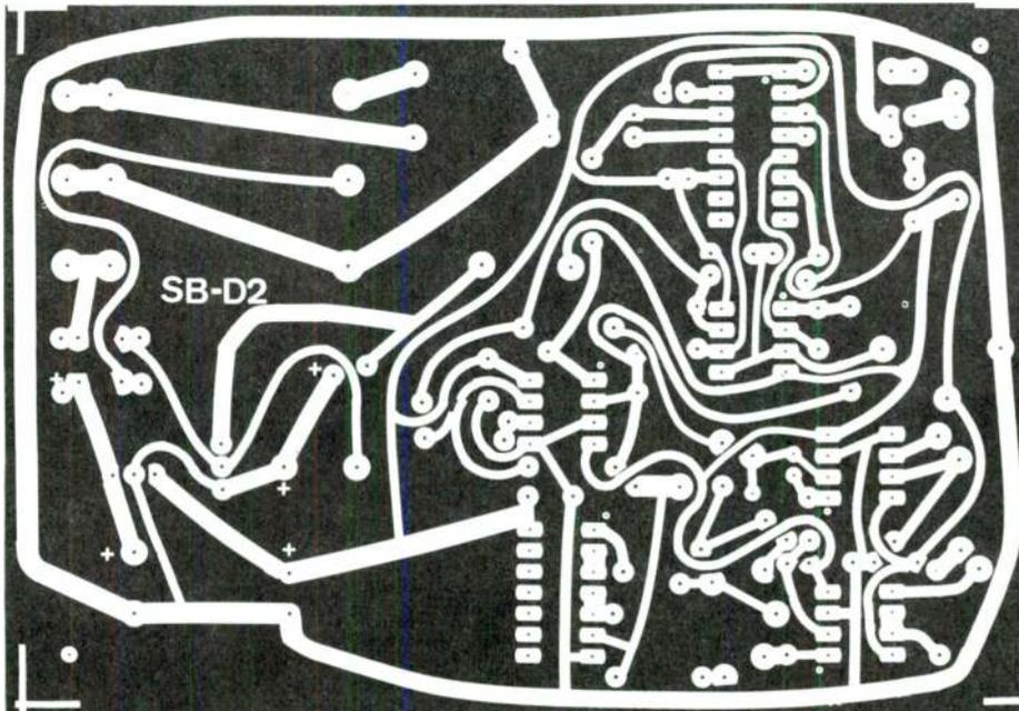
FIGURE 12: Circuit board pattern for the pulse generator.
