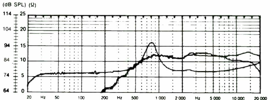
FIGURE 1: The Audax 1-inch tweeter response curves on axis and 30° off axis, as well as its impedance curve.
