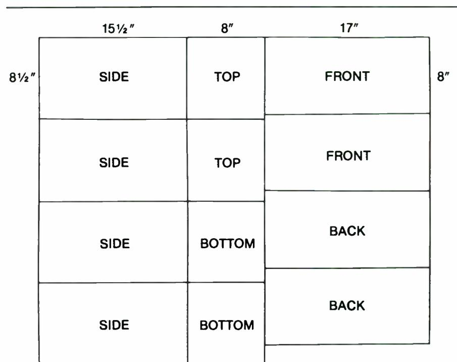
FIGURE 5: Cutting guide for 1/4-inch (18mm) chipboard or plywood.
