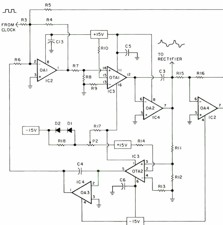
**FIGURE 8:** The schematic for the bandpass filter shows how OTA's instead of resistors provide variable center frequency.
