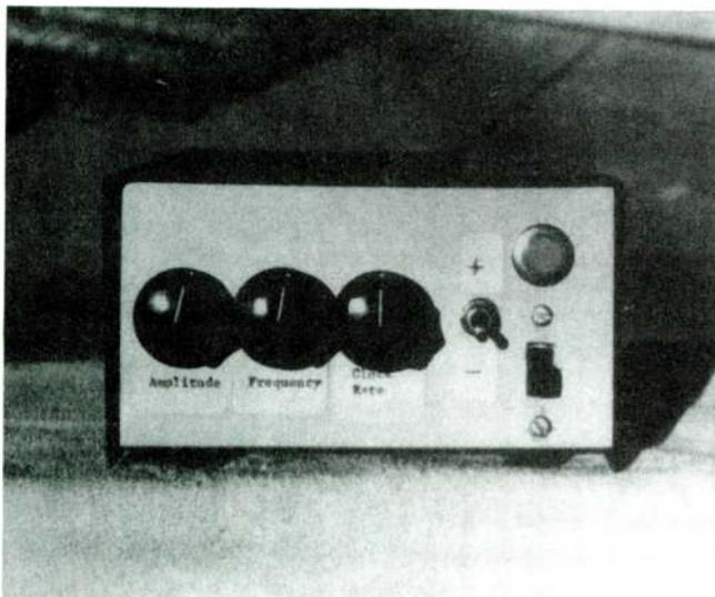
**PHOTO 1:** The front panel has few controls. The frequency pot is a 10 turn type.
