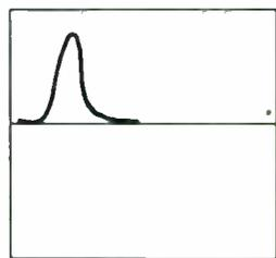
**FIGURE 6:** When the drivers' outputs are in phase acoustically, the pulses in the scope overlap and have maximum amplitude.
