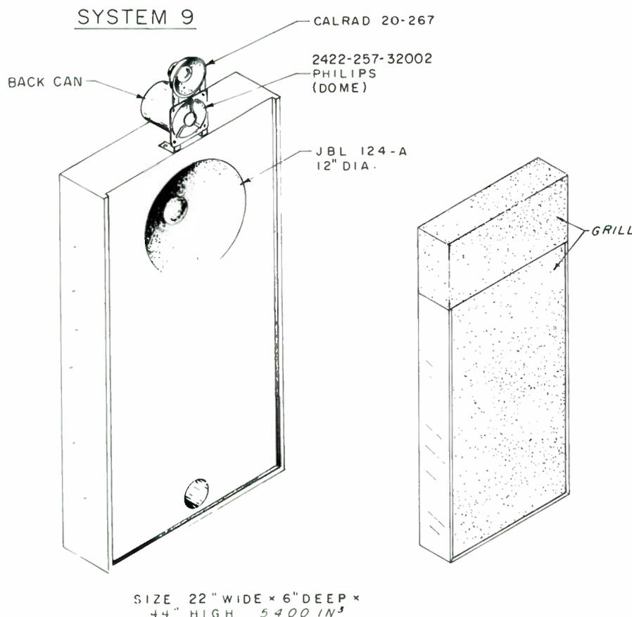
them at some horizontal distance from the rest of the drivers. They would have to be aligned vertically. So, using the former subwoofer cabinet and its newly built twin, I free-mounted the midranges and tweeters to make Full-Range Panels.
