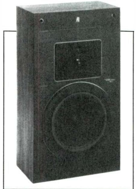
The new **KEF KM-1 Monitor Loudspeaker** features an integral power amplifier with a maximum output exceeding 1,200W. The amplifier is comprised of two power supplies and eight separate output sections to feed seven drive units. Other features include an active three-way dividing/equalizing network, a hybrid floating input circuit and an S-type soft-clipping limiter that is
