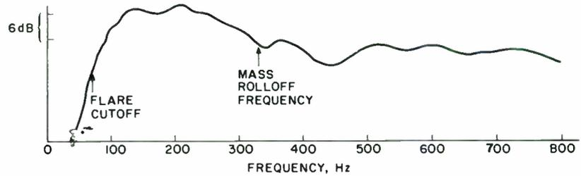
FIGURE 19: System response with the mid-size box extends down to 70Hz.
