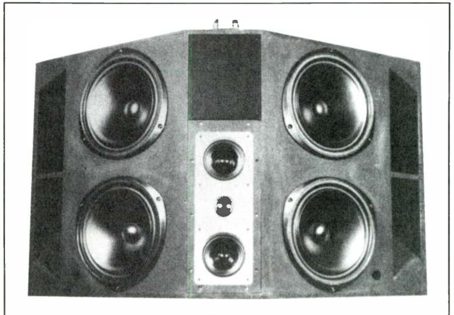
The **NAKAMICHI SP-400** Mobile Speaker System is the last link in the company's complete Mobile Sound System. The three-way speaker's most impressive feature is a separate housing for the crossover networks, which minimizes distortion due to magnetic leakage. The speaker spans a broad frequency range—50Hz to 22kHz—and has a maximum power rating of 80W (40W nominal). Crossovers occur at 2.5kHz and 8.5kHz. Contact Nakamichi USA, 1101 Colorado Ave., Santa Monica, CA 90401.
