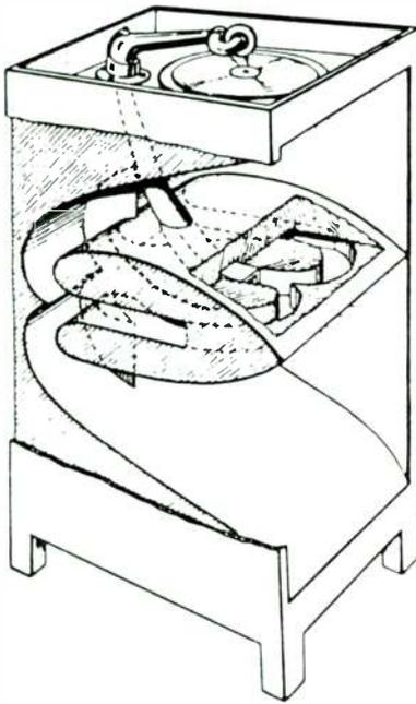
FIGURE 3: RCA's Orthophonic phonograph of 1926 used a folded horn and inspired Edgar's design.
