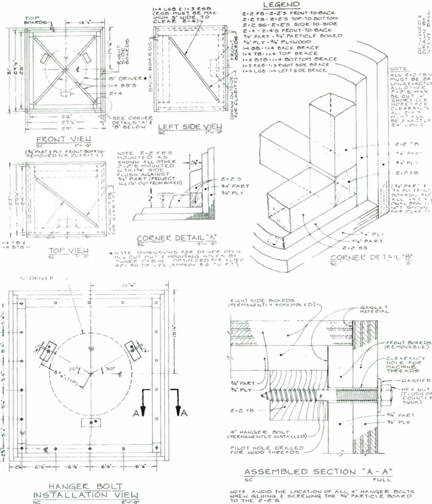
**Figure 3:** The driver and removable front baffle are held into place by three 5-inch and 18 4-inch bolts. On the basis of his experience in building water beds, the author chose these bolts for maximum strength. For additional support, add the optional 2x4's to the P.A. columns.
