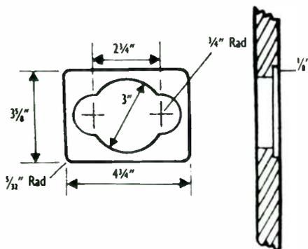
FIGURE 4: Cutout details for the tweeter mounting. Note the 1/8-inch recess, which allows you to flush mount the unit's steel plate.
