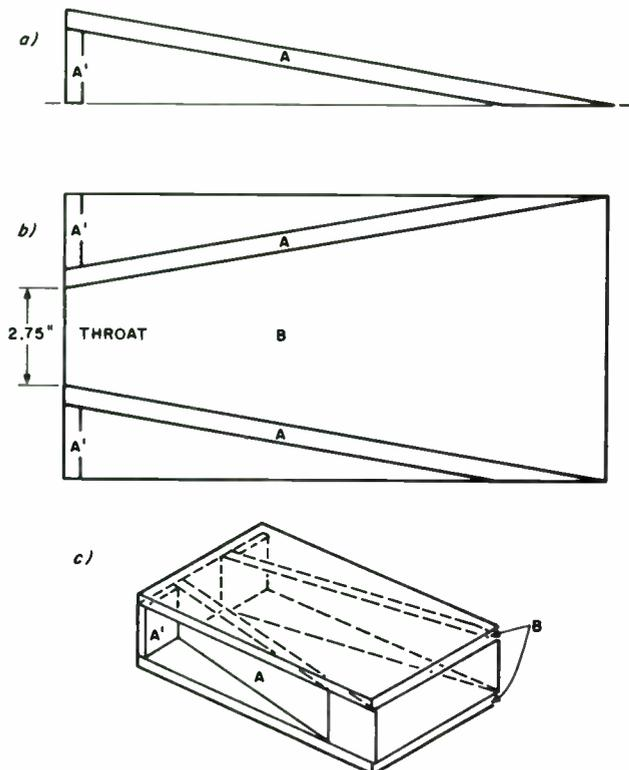
**FIGURE 8:** Begin construction with the throat manifold. The three steps in its assembly are illustrated above.
