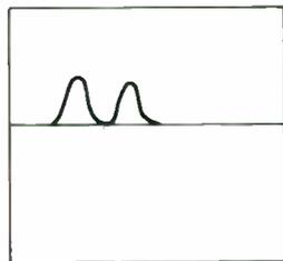
**FIGURE 5:** After rewiring the drivers for the same polarity, adjust the pulse frequency so the amplitudes are equal.
