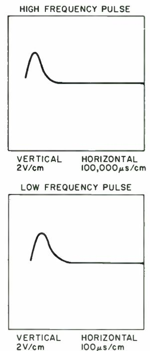
FIGURE 2: Both the HF and LF pulses have the same shape and polarity (positive shown above).
