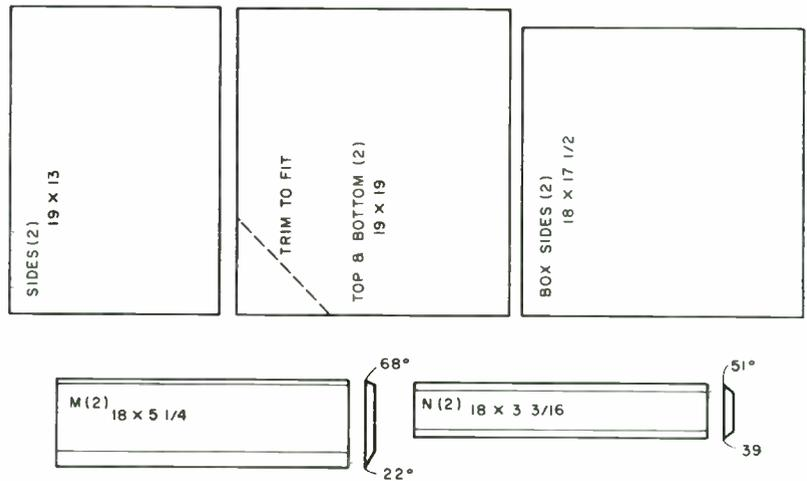
FIGURE 5: The dimensions for all of the particle board parts are as shown. The number needed for one complete horn is circled inside each part.
