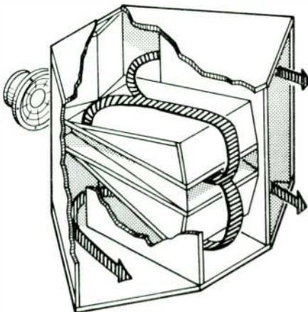
FIGURE 4: The air passages in the 70Hz folded corner horn are similar to the 1926 Orthophonic design.
