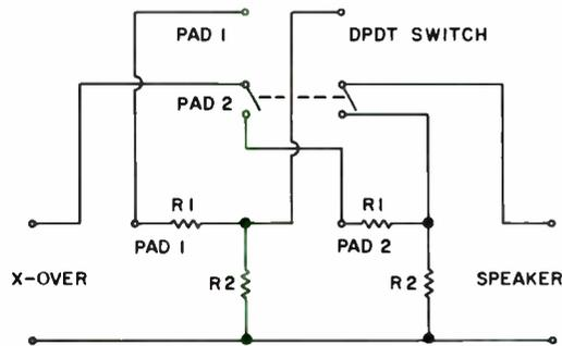
FIGURE 3: Simple switchable L-pad.
