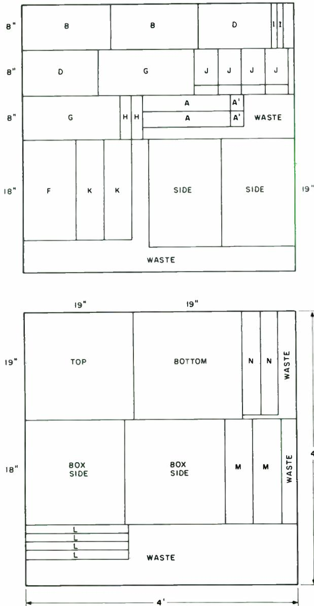
FIGURE 6: For efficient use of the 1/2" plywood or particle board, cut the parts with this pattern.
