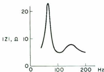
FIGURE 18: With the mid-size box, the resonance is at the right place for smoothest overall response.
