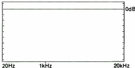
**FIGURE 6:** Frequency versus magnitude of a pulse signal.
