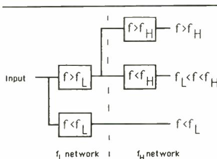
**FIGURE 1:** The block diagram of the cascade connection of a pair of two-way crossovers, forming a three-way network.
