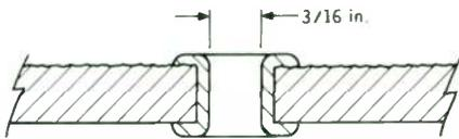
FIGURE 3: Close-up view of a grommet inserted into hardboard.
