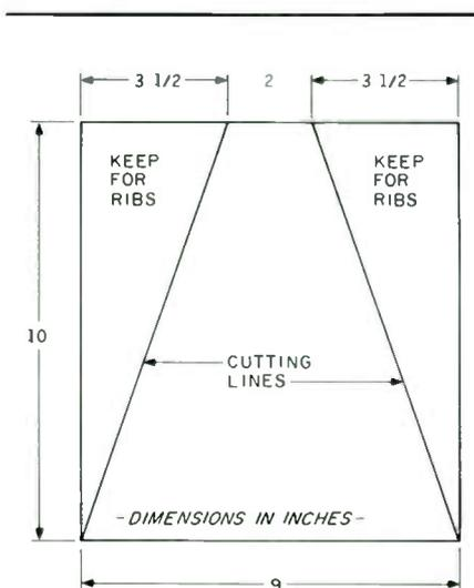
**FIGURE 7:** The cutout diagram for the trapezoidal form used in the horn jig. The form has to be 2 inches thick, and can be made from a sandwich with different thickness boards.
