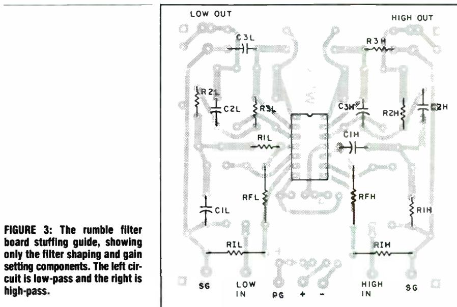
**FIGURE 3:** The rumble filter board stuffing guide, showing only the filter shaping and gain setting components. The left circuit is low-pass and the right is high-pass.
