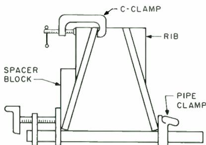
**FIGURE 14:** The clamp arrangement for mounting the ribs.
