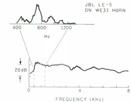
FIGURE 4: The spectrum response of a JBL LE-5 driver on the WE 31 horn. The blown up spectrum on a linear amplitude scale emphasizes the response peaks between 400 and 1200Hz.
