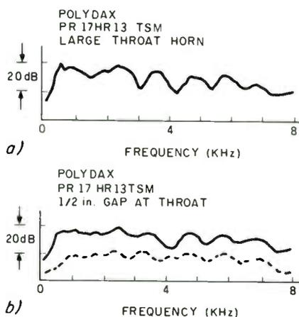
FIGURE 24: Response (a) is of a Polydax PR17HP37TSM 6-inch driver on the large throat horn. Response (b) is the same driver with a 1-inch gap at the throat stuffed with foam at the edges. The free air space response is shown for comparison.
