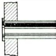
FIGURE 1: The Well-nut is a blind fastener, and can be installed from outside an enclosure.
