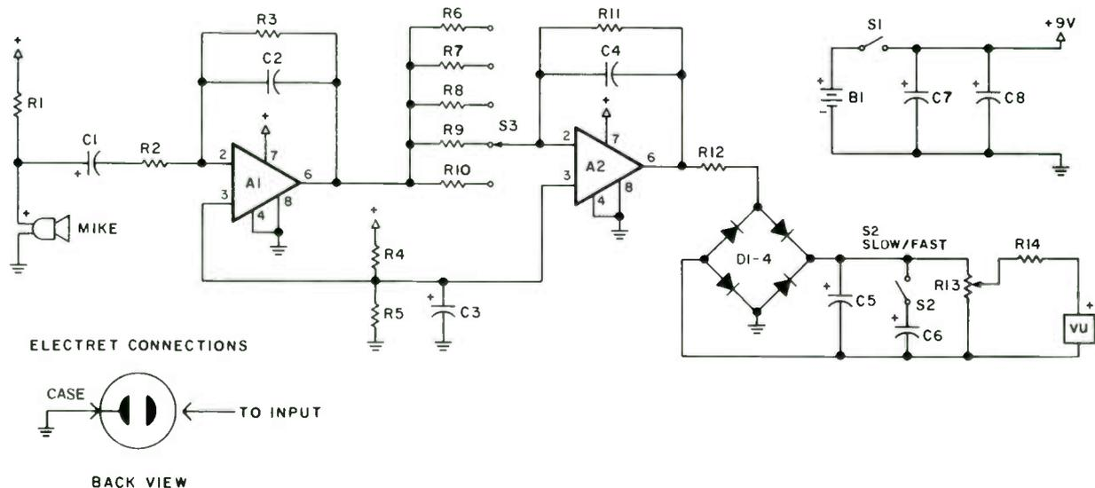
FIGURE 2: Schematic diagram of Mr. Szekeres's sound level meter.
