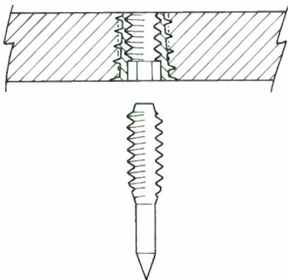
FIGURE 5: The insert is mounted into speaker bases, and the spike is easily screwed in or out for use on different surfaces.
