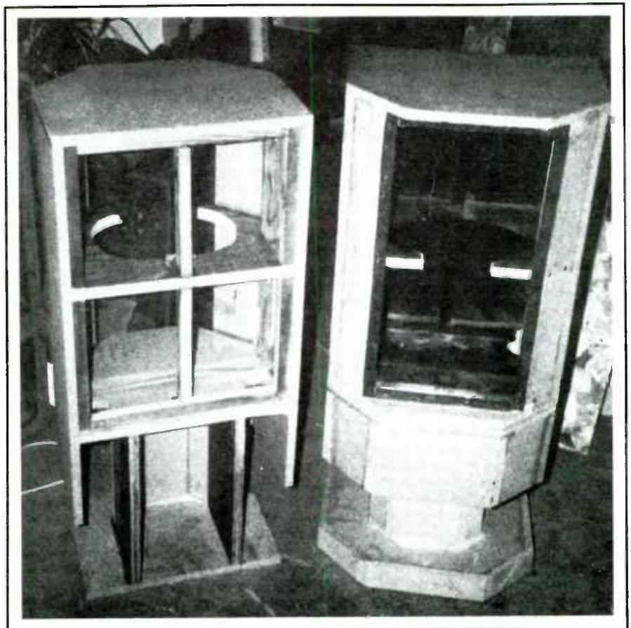
**PHOTO 2:** Cabinet construction front and back. Note bulkhead placement.
