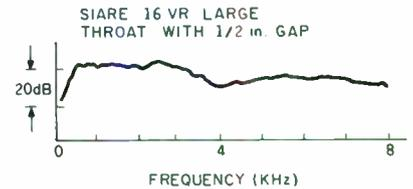
**FIGURE 20:** The response of an SIARE 16VR mounted on the shortened horns with 1/2-inch spacers. Notice the response has smoothed out from those in *Figs 16 and 18*.
