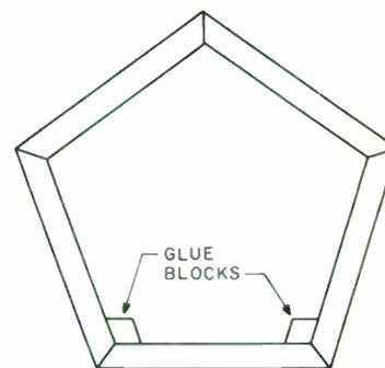
**FIGURE 4:** Position of the first two glue blocks. Be sure the cabinet lies on a flat, smooth surface.
