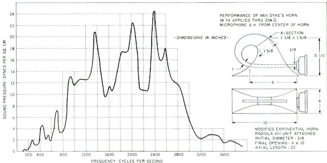
FIGURE 1a: The response of an experimental exponential horn (circa 1924) as measured by an RCA engineer. Notice the prominent response peaks. *Courtesy of the Smithsonian.*
