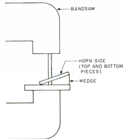
**FIGURE 12:** An alternative method for correctly cutting the beveled edges for the top and bottom pieces.
