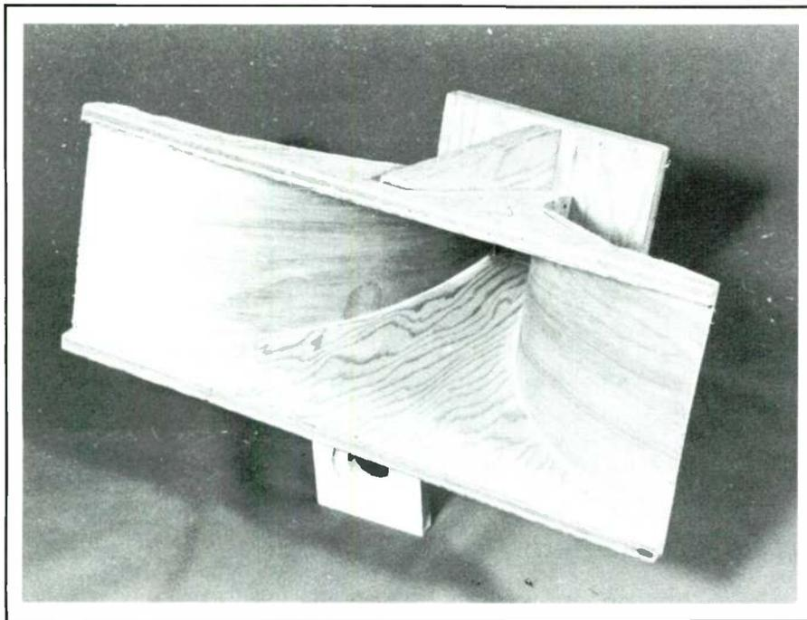
**FIGURE 13a:** An early experimental horn of mine with thin walls of 1/4-inch bent wood.
