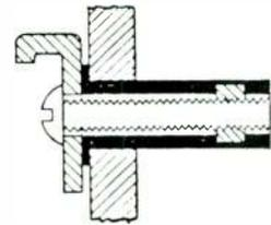
FIGURE 2: The part to be attached is placed against the flange and secured by the machine screw engaging the internal brass nut.
