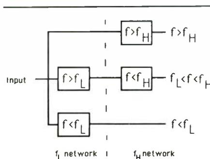
**FIGURE 2:** The parallel connection of a pair of two-way crossovers to form a three-way crossover.
