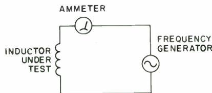
FIGURE 1: Test setup for determining the value of unspecified coils.
