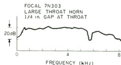
FIGURE 25: The response of a Focal 7N303 7-inch driver on a large throat horn with a 1/4-inch gap at the throat.
