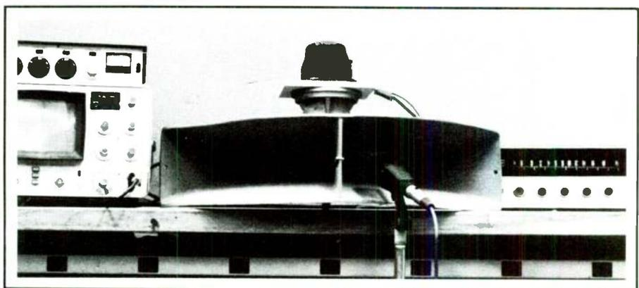
FIGURE 3: The initial test setup using a Western Electric Horn (Model 31), an HP sweeping analyzer, an old Scott receiver, a Shure microphone preamp and a Sennheiser MD-421 microphone.
