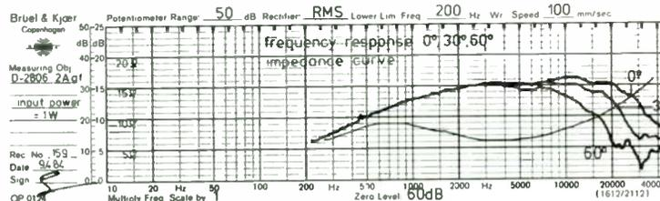
Frequency response from 3,000 up to 40,000 Hz  $\pm 1$  dB!! The impedance curve shows the resonance well damped.
