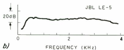
**FIGURE 15:** Response (a) is of a JBL LE-5 driver on 300Hz tractrix horn. Note the nulls at 4 and 7kHz. Response (b) is of (a) on an expanded scale.
