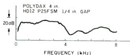
FIGURE 23: The response of the Polydax HD12P25FSM 4-inch driver on the tractrix horn with a 1/4-inch gap at the throat and the gap edges filled with foam.
