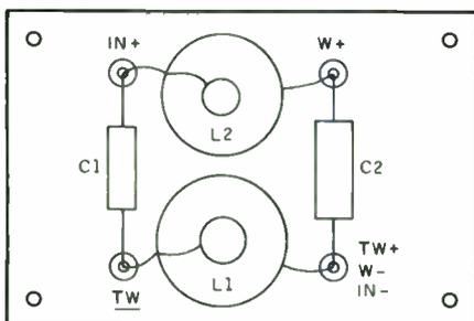
FIGURE 1: I use a "loop" layout for my second order design.
