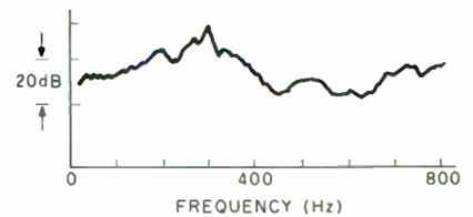
**FIGURE 13b:** The resonant nature of the thin wall horn produced by thumping the horn in front of a microphone. Notice the peak at 300Hz that will color sound.
