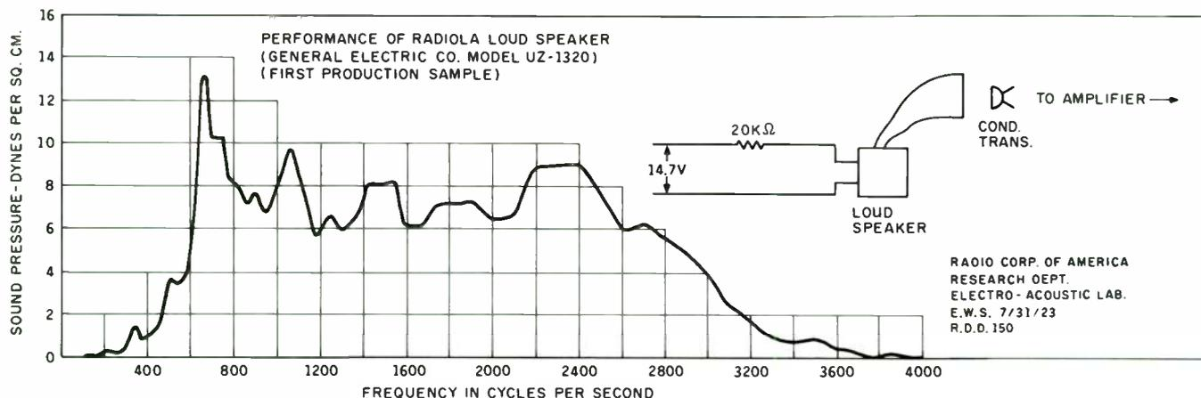
**FIGURE 1b:** The response of a midrange horn as measured by an RCA engineer (circa 1923). Other than the peak at the low end, the response is fairly smooth (less than 3dB ripple). Courtesy of the Smithsonian.
