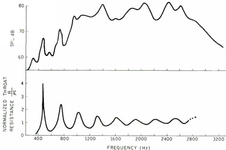
FIGURE 5a: The measured response of the old midrange horn of Fig. 1a, plotted on a log scale, compared with the calculated throat resistance.
