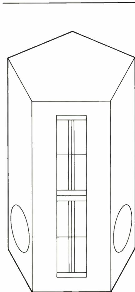
**FIGURE 1:** Bass drivers mounted on side panels will radiate as one at low frequencies.
