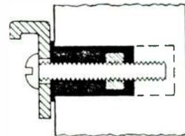
FIGURE 3: As you tighten the screw the neoprene body is compressed, forcing it to tighten behind thin walls (a) or expanding tightly against the walls of a hole (b).
