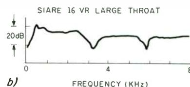
**FIGURE 18:** Response (a) is of an SIARE 16VR on a large throat horn. Note the response peak at the low end (500Hz). Response (b) is of (a) on an expanded scale. Note the nulls in the response are similar to those in Fig. 15.
