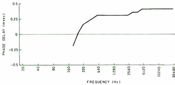
**FIGURE 1: Bessel crossover, zero delay at woofer location.**
