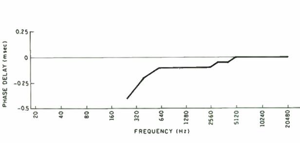
**FIGURE 2: Bessel crossover, zero delay at tweeter location.**
