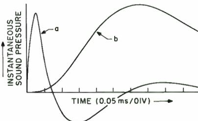
**FIGURE 1: Step response of tweeter (a) and midrange (b) models with ideal third-order crossover.**
