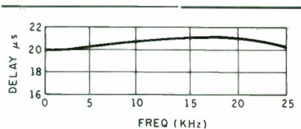
**FIGURE 3:** Simulation of  $20\mu\text{sec}$  delay: modified Pade approximation ( $C=0.85$ ): 5% peaking; cutoff, 27kHz.
