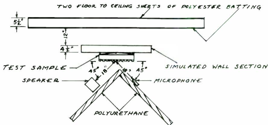
FIGURE 3: Spot sound absorption test setup.
