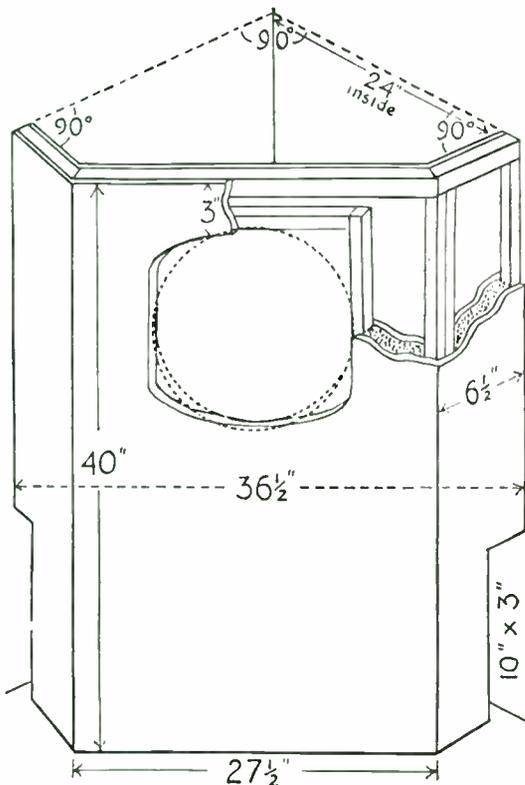
Distance along wall from corner to front of lid is 26 1/4" Weight of front panel 124 lb.
