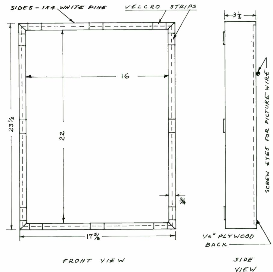
FIGURE 1: Absorber frame construction.
