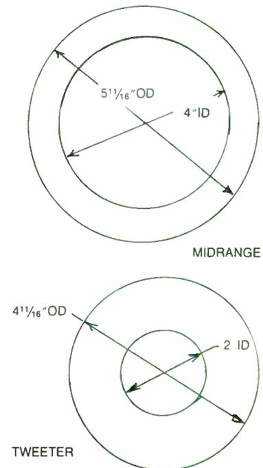
**FIGURE 1:** The midrange and tweeter adapter rings.
