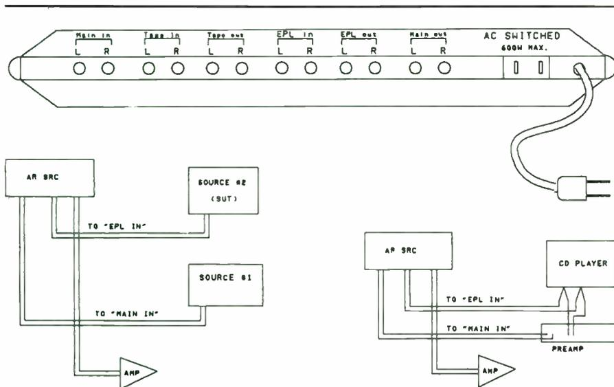
FIGURE 1: The back of the AR-SRC and typical SUT/reference comparison connections.
