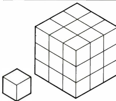
FIGURE 4: Increasing a cube's dimensions three times equals an increase in volume 27 times.
