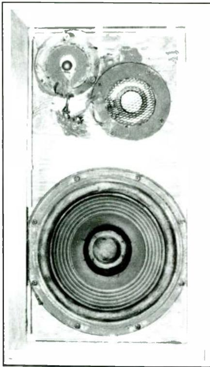
PHOTO 2: The AR-3a with grille removed.
