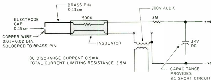
FIGURE 3: STL Ionophone; DC discharge current 0.5mA, total current limiting resistance 3.5M.
