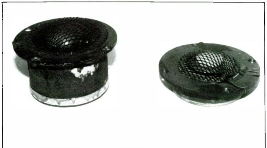
PHOTO 3: The AR-3 midrange (L) as compared to the AR-3a midrange (R).
