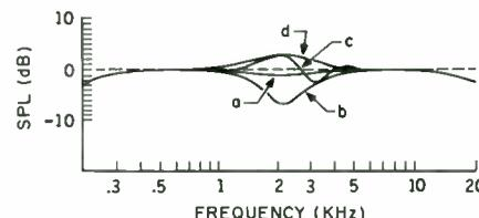
**FIGURE 2: Net frequency response with interdriver time delay: (a) 0mSec, (b) -0.05mSec, (c) -0.375mSec, (d) 0.125mSec.**
