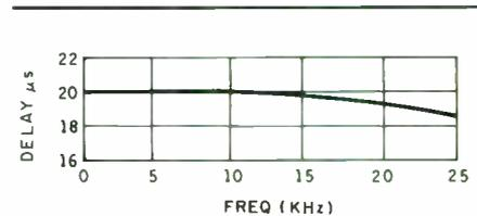
FIGURE 1: Simulation of 20 $\mu$ sec delay: Pade approximation (C=0.68).
