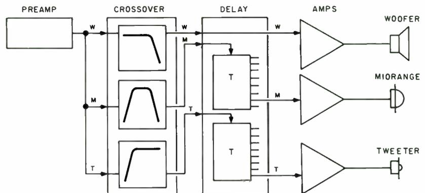
FIGURE 9: Alternate installation location of delay line.
