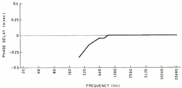
**FIGURE 3: First-order crossover, zero delay at woofer/tweeter location.**
