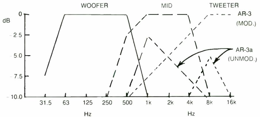
FIGURE 3: Frequency response plot of an original AR-3a versus the modified AR-3.
