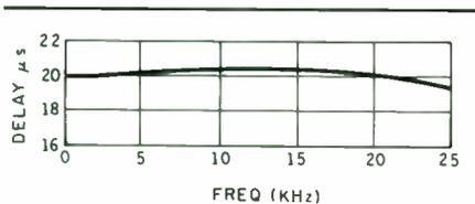
**FIGURE 2:** Simulation of  $20\mu\text{sec}$  delay: modified Pade approximation ( $C=0.75$ ): 1.5% peaking; cutoff, 20kHz.
