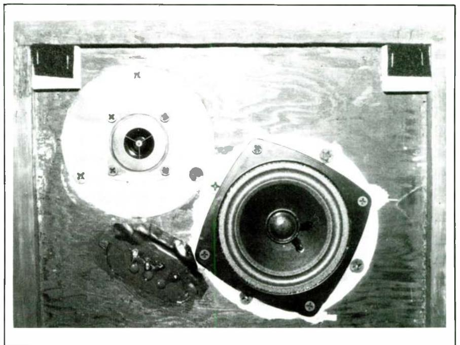
**PHOTO 10:** The Peerless K040MRF and Audax TW51A units installed in the AR-3 box.
