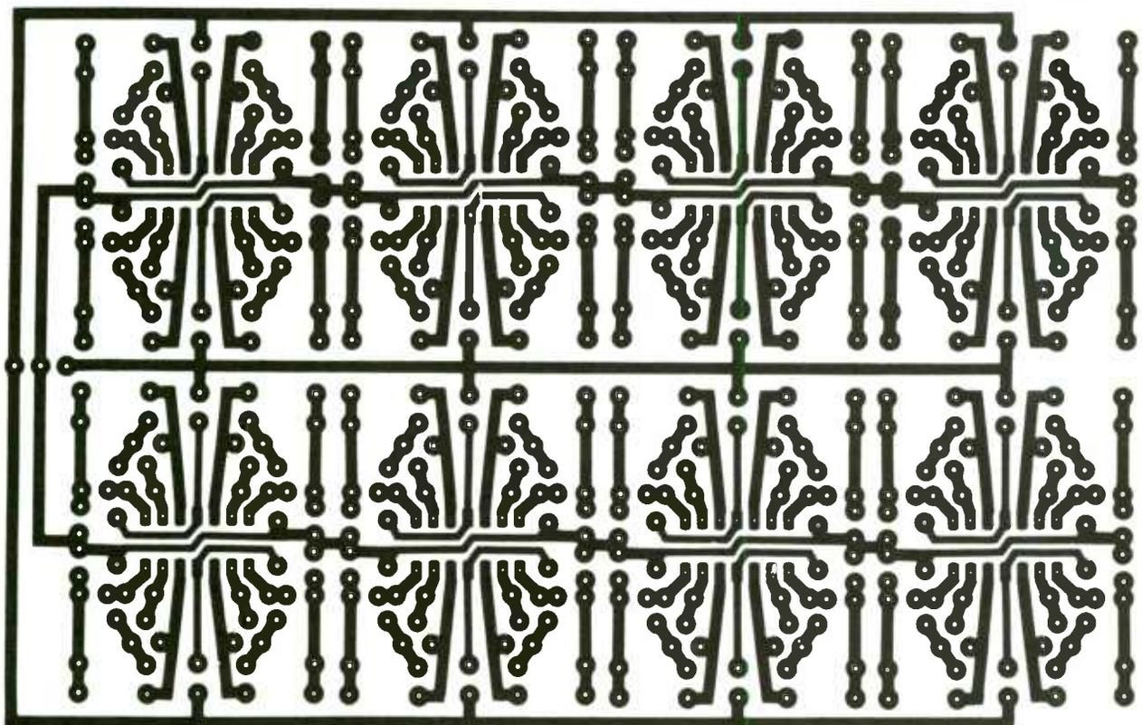
**FIGURE 6:** Circuit board for two channels of 320μsec maximum delay.
