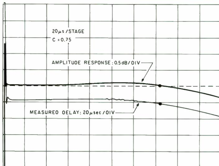
**FIGURE 5:** Measured response of four cascaded  $20\mu\text{sec}$ -delay sections ( $C=0.75$ ).
