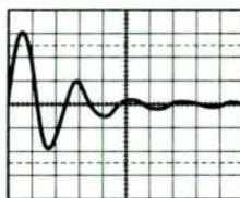
Multiple resonances in a 2 µf capacitor bypassed with an external .22 µf capacitor. Result: high distortion.
