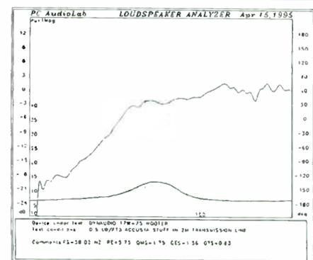
FIGURE 8: PC AudioLab impedance and SPL measurement for 0.5 lb/ft<sup>3</sup> stuffing.
