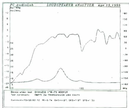
FIGURE 7: PC AudioLab impedance and SPL measurement result for unstuffed transmission line.
