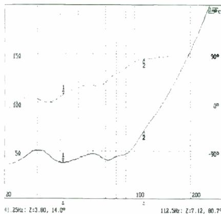
**FIGURE 47:**  $Z_{IN}$  for dual drivers X, rubber throat, full  $\frac{3}{4}L$  extension, and passive crossover/equalizer.
