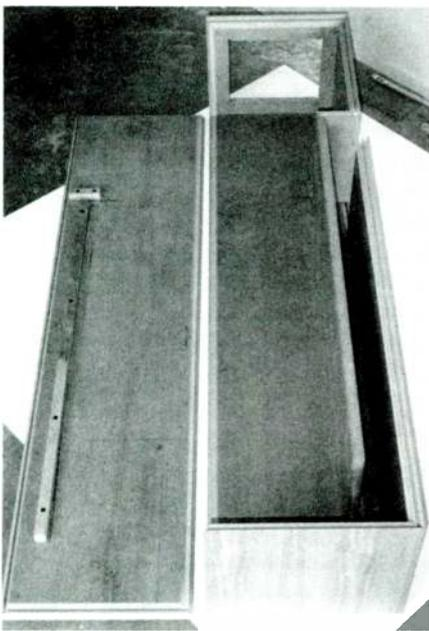
**PHOTO 5:** Cut-away view of middle-section divider in place.
