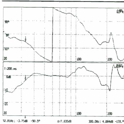
FIGURE 35: Near-field response for dual drivers X with rubber throat, stiffened 9"  $\frac{3}{4}L$  extension.
