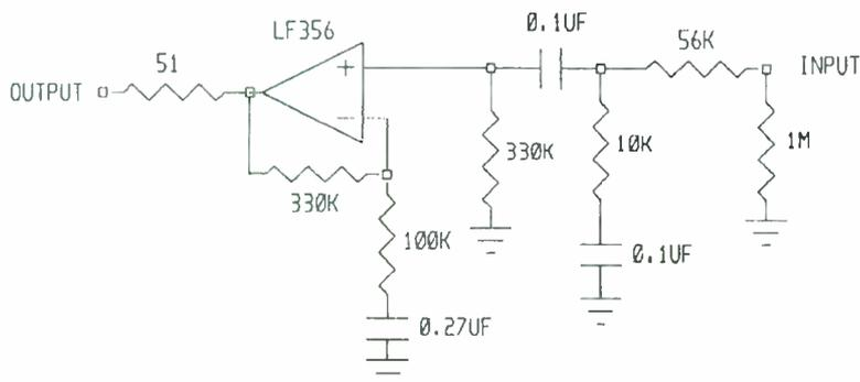
**FIGURE 39:** Schematic for active waveguide equalizer.
