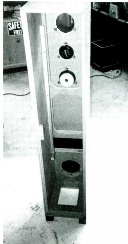
PHOTO 7: Rear view of main TL cabinet, with front faceplate attached.
