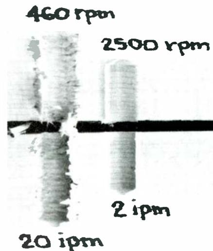
**PHOTO 6:** Effects of drill RPM and feed rates on pilot holes. A larger drill was used to help illustrate the effect.
