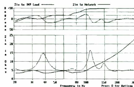
**FIGURE 44:** Computed ZIN to waveguide with passive crossover/equalizer.
