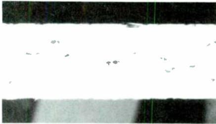
**PHOTO 4:** Cross section of PB. Notice the hard, dense surfaces and the less dense center.
