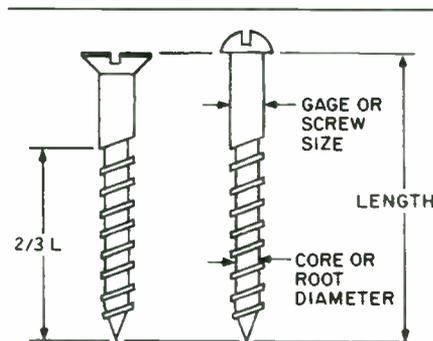
**FIGURE 1:** The parts of a screw.
