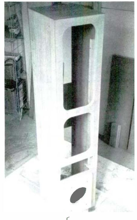
**PHOTO 4:** Assembled main TL cabinet without rear panel attached.
