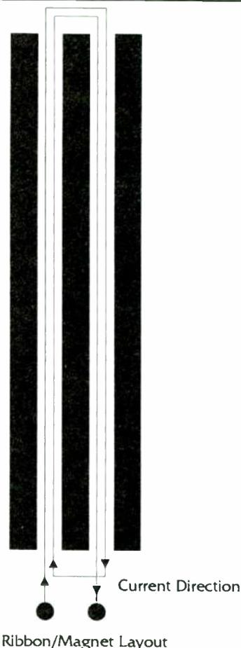
FIGURE 3: Conductor/magnet layout. Keep all current flowing the same direction in each magnetic gap. Two turns with 30 AWG =  $1.6\Omega$ , with 32 AWG =  $2.2\Omega$ , with 34 AWG =  $3.6\Omega$
