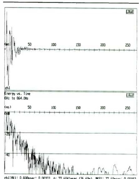
FIGURE 37: Energy-time curve for dual drivers X on modified waveguide.
