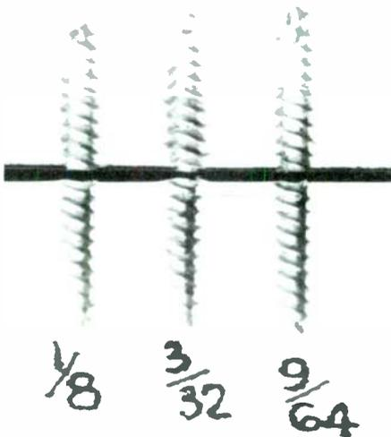
**PHOTO 5:** A study of pilot-hole size in forming good penetration patterns for screws.
