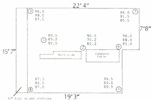
**FIGURE 50:** Basic layout of IMP testing room and SPL levels at various locations.
