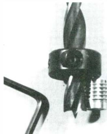
PHOTO 10: Setting the depth of a drill stop for an insert.
