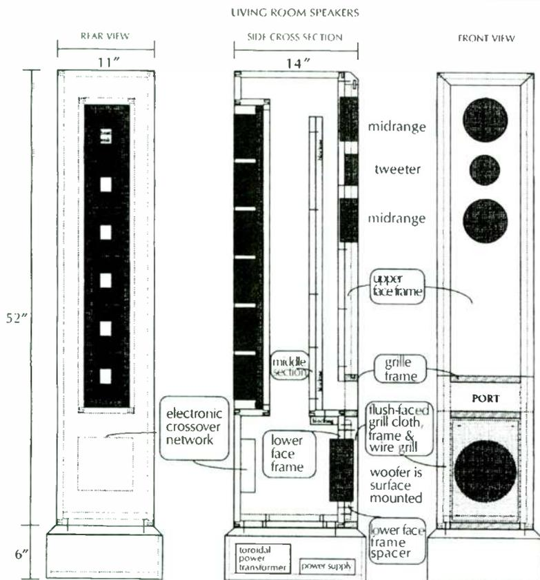
FIGURE 1: Drawing of transmission-line enclosure.
