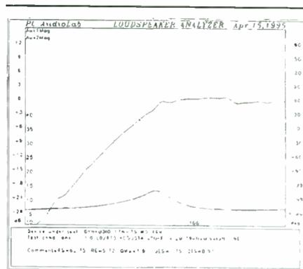
**FIGURE 9:** PC AudioLab impedance and SPL measurement for 1.0 lb/ft<sup>3</sup> stuffing.
