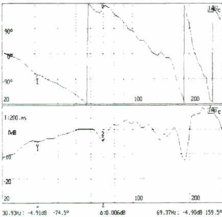
**FIGURE 49:** Near-field response for dual drivers X in series with rubber throat and full  $\frac{3}{4}L$  extension.
