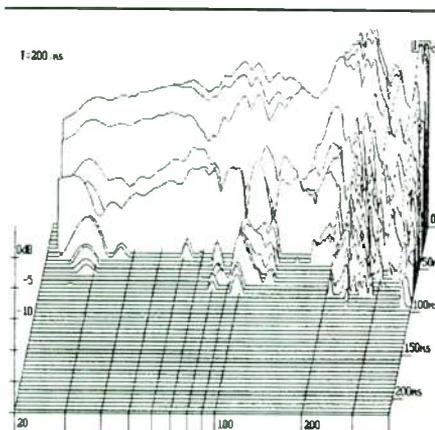
FIGURE 34: Waterfall plot for dual drivers X with rubber throat, stiffened full  $\frac{3}{4}L$  extension.
