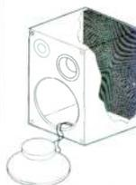
Place the flexible Deflex panel thru' the speaker cut-out and stick to the inside of the cabinet using the recommended adhesive
