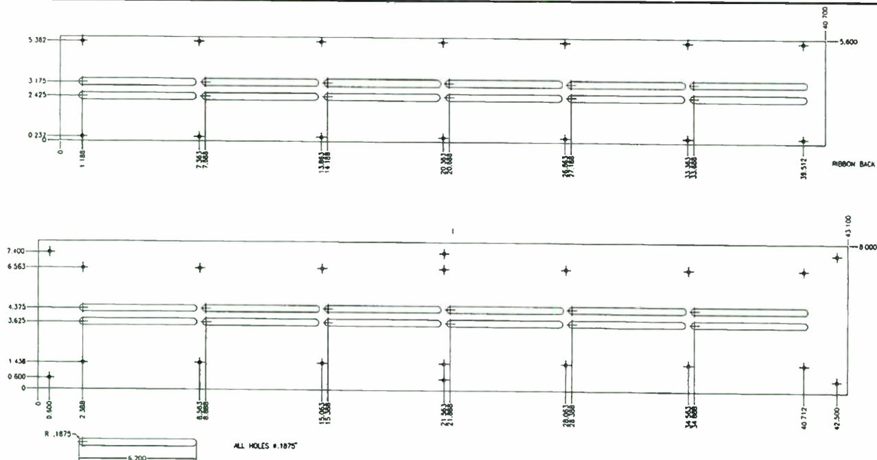
**FIGURE 1:** Front and rear plates.
