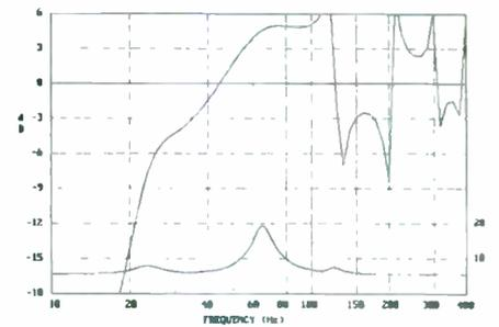
**FIGURE 2:** TLBOXMODEL impedance and SPL result for 0.1 lb/ft<sup>3</sup> stuffing.
