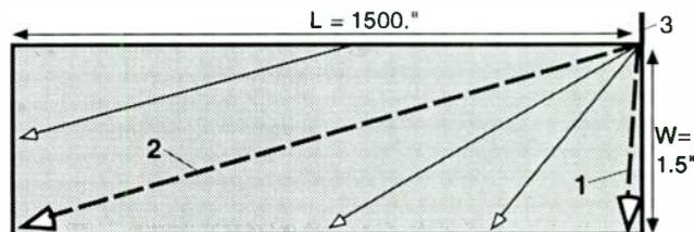
Your capacitors have another problem that's even worse. They roll up signal path 2 into a tight corkscrew coil (below). The inductance of any coil is multiplied by the number of turns squared, and there can be 1000 turns in an audio capacitor. So the inductance of path 2 can be a million times higher than straight path 1, delaying music a million times worse for some paths through the capacitor than for other paths. This capacitor actually smears music by a factor of 1,000,000:1.
