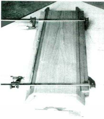
PHOTO 6: Assembly of front faceplate.
