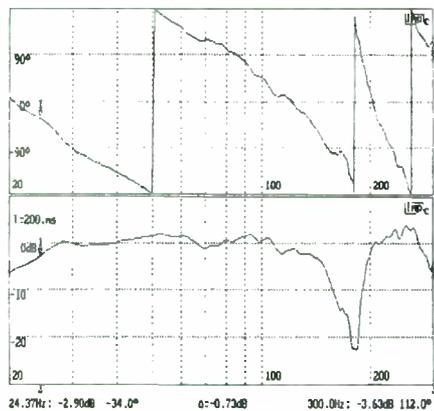
**FIGURE 42:** Near-field response dual drivers X, rubber throat, full 3/4L extension, and active equalizer.
