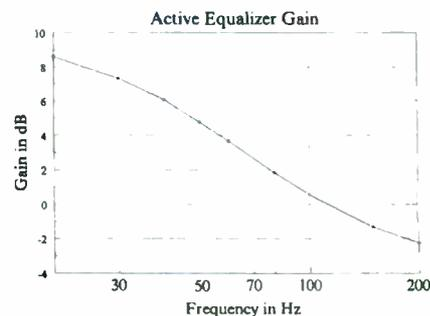
**FIGURE 40:** Measured response of active equalizer.
