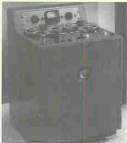
Out of the Mullin-Palmer Magnetaphon developments, came Ampex models 200, April 1948, 300 (shown), 400 and station favorite, the 350 debuting in 1954 with more than 40,000 units produced.
