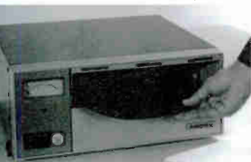
The Ampex AG100 Cue-Mat is basically a slab of oxide using analogue technology. It could be considered one of the numerous experiments leading to the floppy disc.
