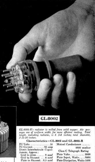
Use of center-tapped filaments permits paralleling of filament leads for low inductance r-f feed. Reduced ratings permit operation up to 200 mc air-cooled, 300 mc water-cooled.
