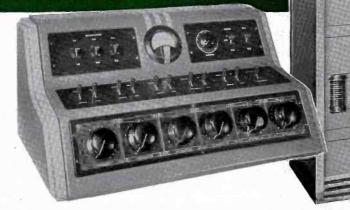
RCA 78-B1 operator's console control with switches for connecting preamplifier inputs to microphones in either of two studios, and mixer-outputs to either broadcast or auditioning channels. Other mixing circuits for turntables and remote lines. Illuminated V.I. meter may be set for either peak or RMS level or a VU meter is available if desired. 78-C1 is similar, but equipped for a single studio only, with 3 input channels but without audition keys.
