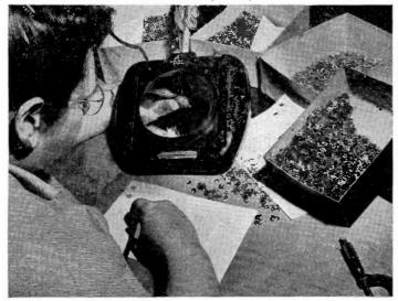
Tiny tube parts are magnified and their outlines superimposed on scale drawings to insure meeting the extremely close tolerances required.
