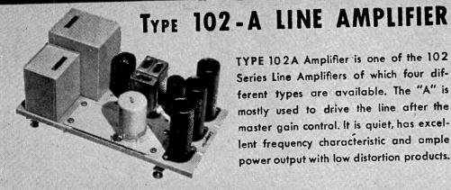
TYPE 102A Amplifier is one of the 102 Series Line Amplifiers of which four different types are available. The "A" is mostly used to drive the line after the master gain control. It is quiet, has excellent frequency characteristic and ample power output with low distortion products.
