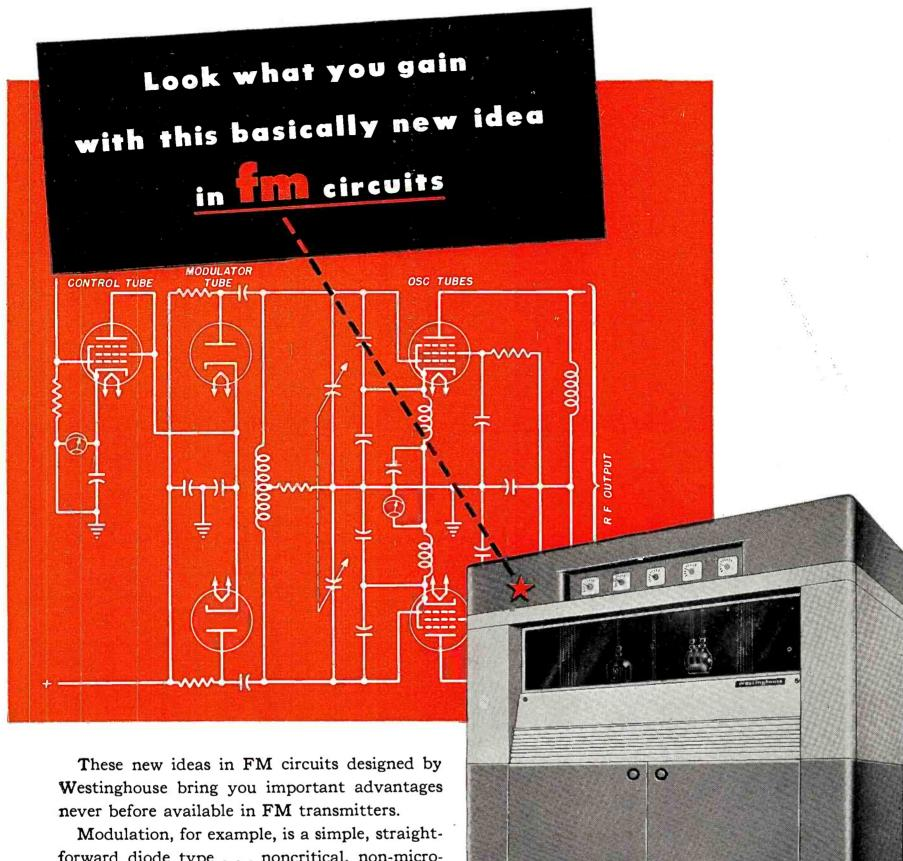
forward diode type . . . noncritical, non-microphonic, no-trick tubes (see drawing above). The effective resistance of the tubes is a function of plate current in the modulator-control tube.
