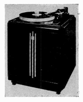
NEW studio transcription table (No. 524) of Fairchild Camera & Instrument Corp., Jamaica, N. Y., is pictured above. Using the Fairchild two-speed drive and synchronous motor with clutch for smooth starting and stopping and shifting speed (without shutting off the motor), the unit provides space and facilities for mounting standard pickups of broadcast quality. Cabinet is of wood.
