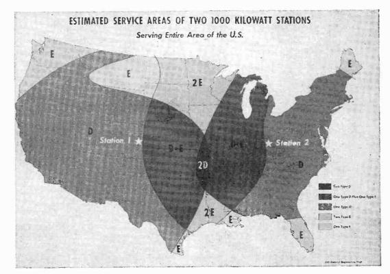
TO SERVE areas not covered by FM networks, CBS said two million-watt AM stations might provide nighttime skywave coverage as shown above, with daytime service from strategically located stations of less power but with extensive groundwave propagation. Symbol "D" refers to bestquality skywave service; "E", second grade. Map contemplates use of 1,000 kc but CBS said this "is not significant." Sites suggested for the high-powered stations were "eastern Colorado" and "northern Kentucky."
