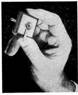
MIDGET five-plate square stack selenium rectifier to replace rectifier tubes in portable radios has been designed by Federal Telephone & Radio Corp., manufacturing affiliate of IT&T. Known as type 403D-2625, unit is composed of five square selenium plates made on aluminum base plates, connected in series and with center contact. Unit measures 1½ x 1½ x 11/16 inches, permitting installation in spaces too small for ordinary tube used for that purpose.
