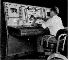
**COMPLETENESS** In television, G-E equipment covers every phase of station operation, from camera channels to transmitters and antennas. Pictured here is the Master Control Desk, an exclusive G-E development
