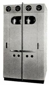
Feedback designed by Bell Laboratories does away with need for hum suppression circuits – maintains flat frequency response.
