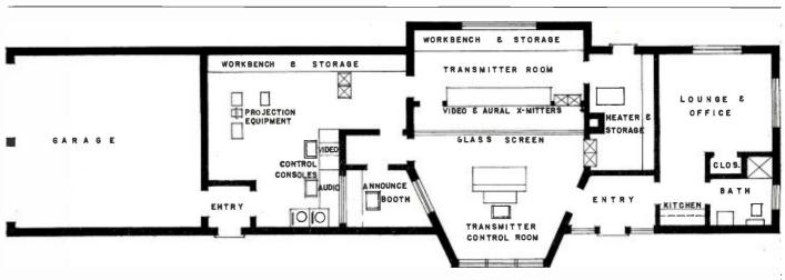
Fig. 1: SUGGESTED plan for housing television transmitter and film projection facilities.
