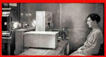
First Television "Camera." As light from electric are at left is projected through 48 fioles of revolving disc, the floshes ore picked up by 4 electric eyes protruding from wooden frame on table. The impulses are then broadcost much the same as any radio message
