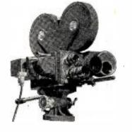
THE MAURER 16MM., designed specifically for professional use, equipped with precision high-power focusing and view-finder. Standard equipment includes: 235° dissolving shutter, automatic fade control, view finder, sunshade and filter holder, one 400-foot gear-driven film magazine, a 60cycle 115-volt synchronous motor, one 8-frame handcrank, power cable and a lightweight carrying case.
