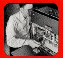
Repid focus by crank or knob. Use inside coupling knob (above) for focus cluster (lines up)
