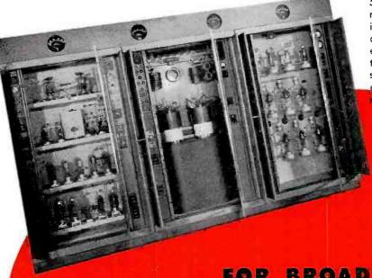
The CONTINENTAL Type 315 Transmitter, at left, offers a deluxe design for 5 KW AM operation. It has many features not ordinarily incorporated in transmitters of this class, including special equipment for matching transmitter output into sharply tuned loads often encountered in directional darrays.
