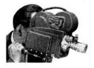
Photograph a sound track along one edge of your picture film with the Auricon "Cine-Voice" 16 mm Camera. Same film cost as old-fashioned silent movies! Edit your own talking pictures on any make of 16 mm sound projector.
