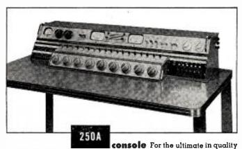
control the 250A Console is the finest unit ever made for AM, FM or TV studio use. Its compactness is made possible by the use of newly designed miniature plug-in preamplifiers, line amplifiers and power supplies. The preamps are only 1 % "x4¼ "x9". The line amplifiers and power supplies are 2%"x4¼"x9". You will find that the new Altec 250A Console leads to better control, more economical operation.
